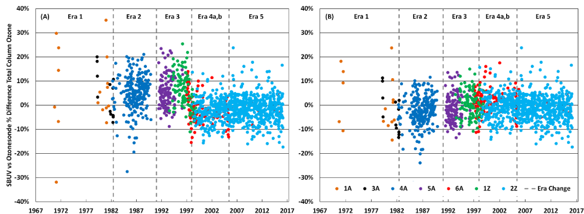
Figure S7: Boulder, CO SBUV vs Ozonesonde total column ozone comparison before (A) and after (B) applying ozone sensor efficiency.
