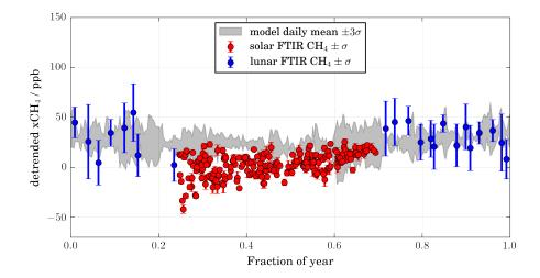
Figure 14. Comparison of solar and lunar xCH<sub>4</sub> FTIR measurements (green dots). Errorbars show  $1\sigma$  standard deviation of the daily mean. The lunar data points have been averaged over one full moon period each. The shaded gray area shows the  $1\sigma$  standard deviation of the MACC CH4 model daily means as shown in Fig. 12.
