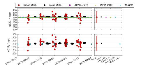
Figure 9. Comparison of the solar and lunar measurements of  $xCO_2$  and  $xCH_4$ in September 2013 (dots) and the corresponding arithmetic means (lines). Values are given in Table 2.
