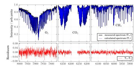
**Figure 2.** Example fit of a measured spectrum (black line) on October 25 2015, the corresponding calculated spectrum (blue line) and their residuum (red line) for the retrieved windows of O2, CO<sub>2</sub> and CH<sub>4</sub>.
