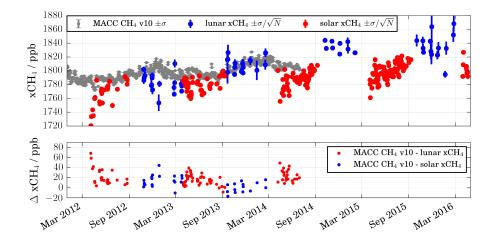
Figure 12. Comparison of the daily means of lunar (blue) and solar (red) xCH<sub>4</sub> FTIR measurements to the AK-smoothed MACC CH<sub>4</sub> model v10 (gray). Errorbars show the standard error ( $\sigma/\sqrt{N}$ , with N number of measurements). The lower panel shows the difference model - measurement.
