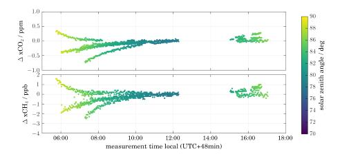
**Figure 4.** Same as Fig. 3 but for TCCON solar absorption measurements for the time between 2013-09-19 and 2013-09-24. Note the generally higher differences at high zenith angles. Between 12:30 and 15:00 local time the sun moves behind a mountain at lower zenith angles.
