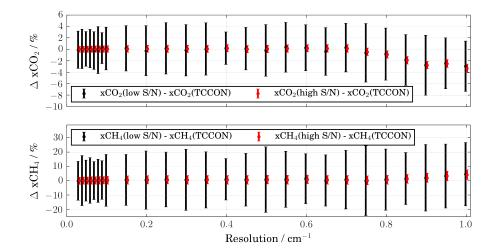
Figure 6. Mean of the retrieved  $xCO_2$  and  $xCH_4$  from cropped interferograms at different resolutions with low and high signal-to-noise ratio. Shown is the relative difference to the highest signal-to-noise ratio and highest resolution. Errorbars show the  $1\sigma$  standard deviation of the mean.
