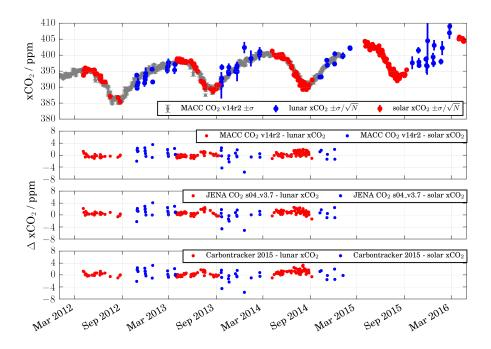
Figure 11. Comparison of the daily means of lunar (blue) and solar (red)  $xCO_2$  FTIR measurements to the AK-smoothed MACC  $CO_2$  model v14r2 (top panel, gray). Errorbars show the standard error ( $\sigma/\sqrt{N}$ , with N number of measurements). The lower panels show the difference model - measurement for all models.
