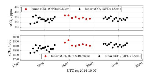
Figure 7. Comparison of retrieved  $xCO_2$  and  $xCH_4$  for different resolutions from low (**OPD** = 1.8 cm=0.5 cm $^{-1}$ , black) and higher (**OPD** =  $10.59 \text{ cm} = 0.085 \text{ cm}^{-1}$ , red) resolution measurements on 2014-10-07.
