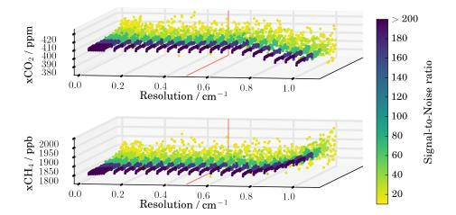
Figure 5. Retrieved  $xCO_2$  and  $xCH_4$  from cropped interferograms with different resolutions and different levels of white noise (z-axis and colorbar) added to the spectra.
