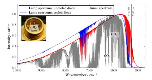
**Figure 1.** Example measurements of the InGaAs diode: Cooled (blue) and uncooled (red) lamp spectra. Note the indication of the cut-on wavenumbers. An averaged lunar spectrum is shown in gray and a picture of the diode was added.
