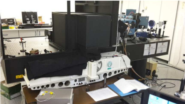
Figure 3: Photo of the CMI measurement setup. Double-grating monochromator is on the left side, the output optics light-tight box in the middle of the picture as well as the Dobson 074.
