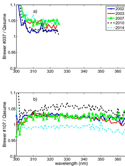
**Figure 10.** The results of the comparisons between (a) Brewer #037, (b) Brewer #107 and the QASUME during 2002–2014. The irradiances of the Brewers were cosine error corrected.
