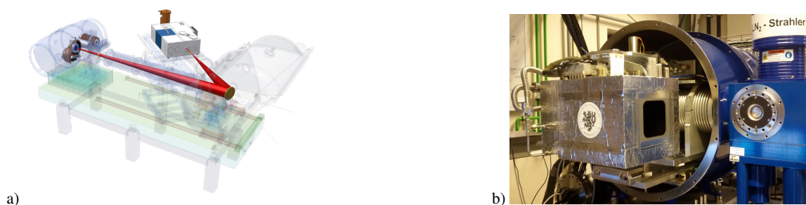
Figure 5. (a) The Reduced Background Calibration Facility (RBCF) at PTB and (b) The large-area balloon blackbody inside the source chamber of the RBCF
