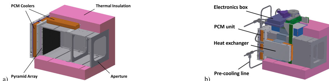
Figure 3. Design of Balloon Blackbody (a) with electronics and heat exchangers for precooling (b)
