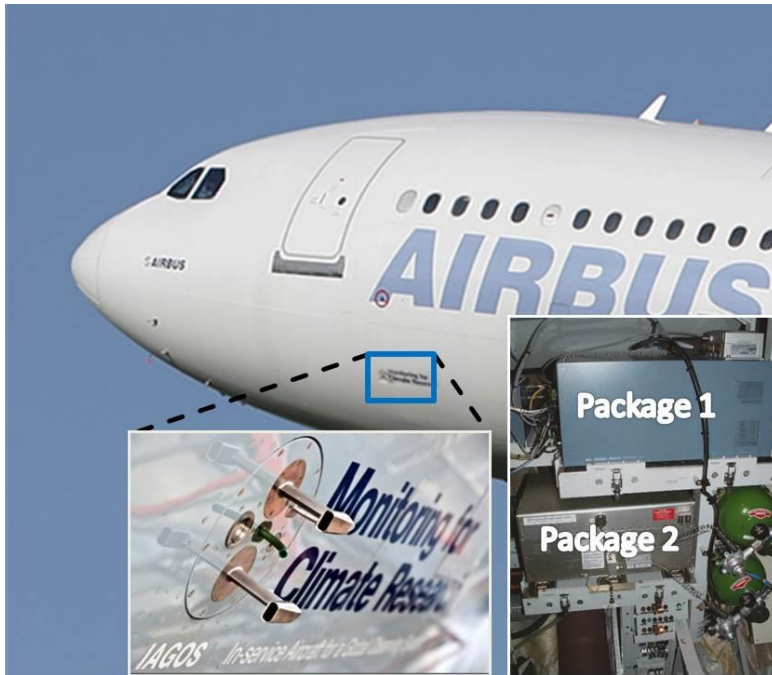
Figure 1: Position of Package 1 and Package 2 installed aboard the AIRBUS A340-300. The inlet plate including the Rosemount housing is attached at the aircraft skin.
