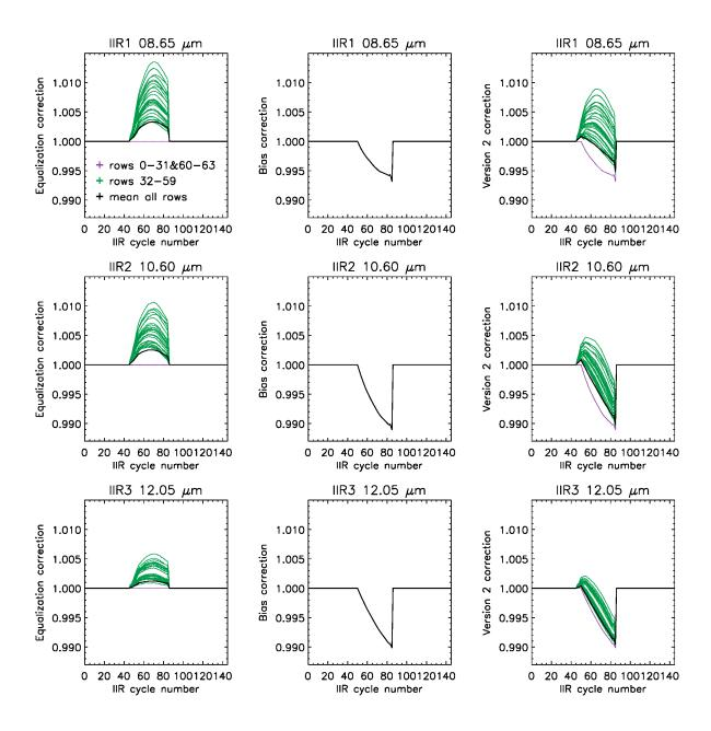
Figure 9: Version 2 correction coefficients applied to Version 1 calibrated radiances (top: IIR1, middle: IIR2; bottom: IIR3) vs. IIR 5 cycle number for each of the 64 rows. Left: equalization correction C<sub>eq</sub>(i,c,k); center: bias correction C<sub>bias</sub>(i,c,k); right: Version 2 correction, i. e. the product of the equalization and bias corrections. Purple: sound rows; green: flawed rows. The black curve represents the mean correction in an image.
