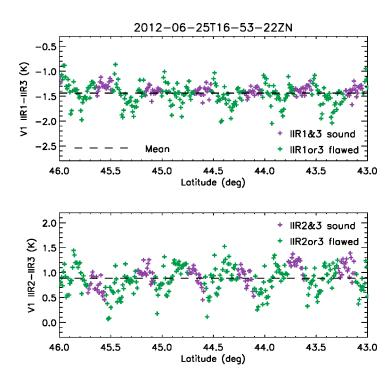
Figure 5: Version 1 IIR1-IIR3 (top) and IIR2-IIR3 (bottom) inter-channel BTDs along the CALIOP track for the same cloud-free scene over water surface on 25 June 2012 as in Fig. 1. Purple: sound rows in both channels; green: flawed rows in at least one channel. Horizontal dashed line: mean value.
