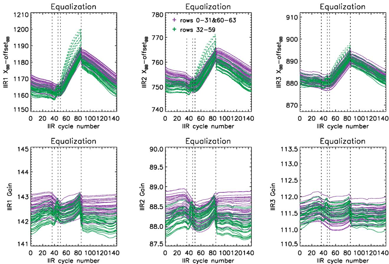
5 **Figure 7: Mean digital counts in offset-corrected blackbody views after equalization correction (top) and resulting mean gains (bottom) vs. IIR cycle number in June 2012 for each of the 64 rows in IIR1 (left), IIR2 (middle), and IIR3 right). Purple: sound rows; green: flawed rows. The dashed green lines in the upper plots show the flawed rows before correction (cf Fig. 4).**
