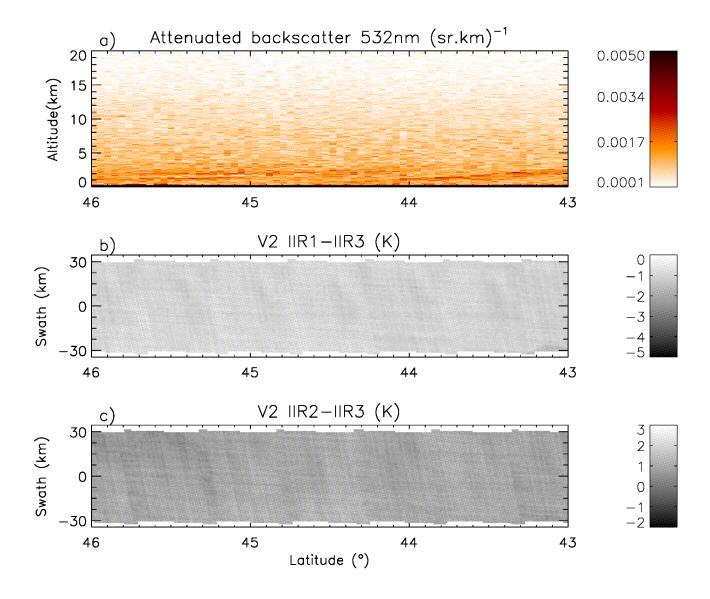
Figure 10: Version 2 IIR inter-channel BTDs in the same nighttime descending portion of the same orbit as in Fig. 1. (a): CALIOP lidar attenuated backscatter; (b): IIR1-IIR3 BTD; (c): IIR2-IIR3 BTD. The striping effect is significantly attenuated compared to Version 1.
