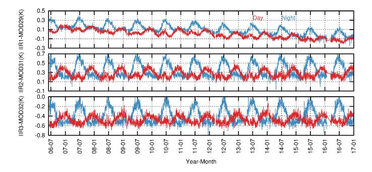
Figure 2: Time series of IIR Version 1-MODIS C5 daily average BTDs over oceans for IIR1-MODIS29 (top), IIR2-MODIS31 5 (middle) and IIR3-MODIS32 (bottom). Latitude range: 30° N-60° N. Temperature range: 280-290 K. Unexpected seasonal differences are seen between nighttime (blue) and daytime (red) BTDs. Adapted from Garnier et al. (2017).
