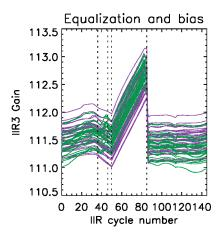
Figure 8: Mean gains vs. IIR cycle number in June 2012 for each of the 64 rows in IIR1 (left), IIR2 (middle), and IIR3 (right) after equalization and bias corrections. Purple: sound rows; green: flawed rows.
