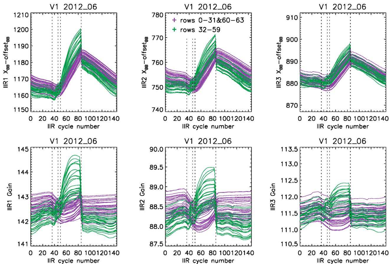
5 **Figure 4: Mean digital counts in offset-corrected blackbody views (top) and resulting gains (bottom) vs. IIR cycle number in June 2012 for each of the 64 rows, showing a different behavior for the purple ( $i=0-31$  and  $60-63$ ) and the green ( $i=32-59$ ) rows. Digital counts and gain are plotted for the three channels: IIR1 (left), IIR2 (middle), and IIR3 (right).**
