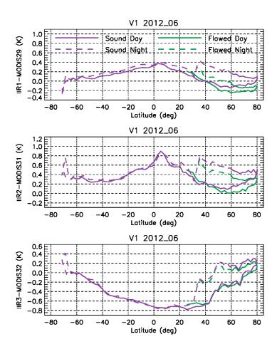
Figure 6: Median IIR Version 1-MODIS C5 BTDs vs. latitude in clear sky conditions over oceans in June 2012. Top: IIR1-MODIS29; middle: IIR2-MODIS31; bottom: IIR3-MODIS32. Purple: sound rows; green: flawed rows. Solid: day; dashed: night.
