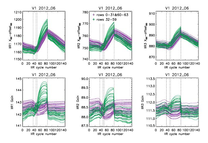
Figure 4: Mean digital counts in offset-corrected blackbody views (top) and resulting gains (bottom) vs. IIR cycle number in June 2012 for each of the 64 rows, showing a different behavior for the purple (i=0-31 and 60-63) and the green (i=32-59) rows. Digital counts and gain are plotted for the three channels: IIR1 (left), IIR2 (middle), and IIR3 (right).
