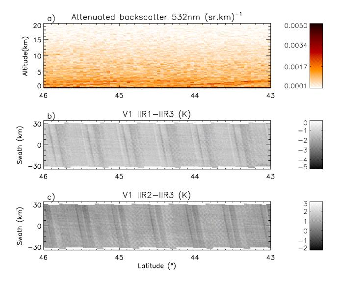
Figure 1: Example of striping effect seen in Version 1 IIR inter-channel BTDs for a cloud-free scene over water surface in the nighttime descending portion of an orbit between 46° N and 43° N on 25 June 2012; (a): CALIOP lidar attenuated backscatter; (b): IIR1-IIR3 BTD; (c): IIR2-IIR3 BTD.
