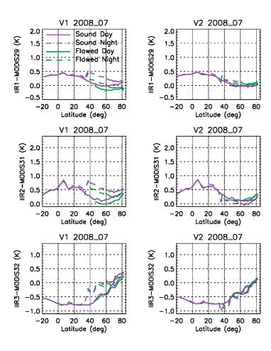
Figure 12: Median IIR-MODIS C5 BTDs vs. latitude in clear sky conditions over oceans in July 2008 for IIR Version 1 (left) and Version 2 (right). Top: IIR1-MODIS29; middle: IIR2-MODIS31; bottom: IIR3-MODIS32. Purple: sound rows; green: flawed rows. Solid: day; dashed: night.
