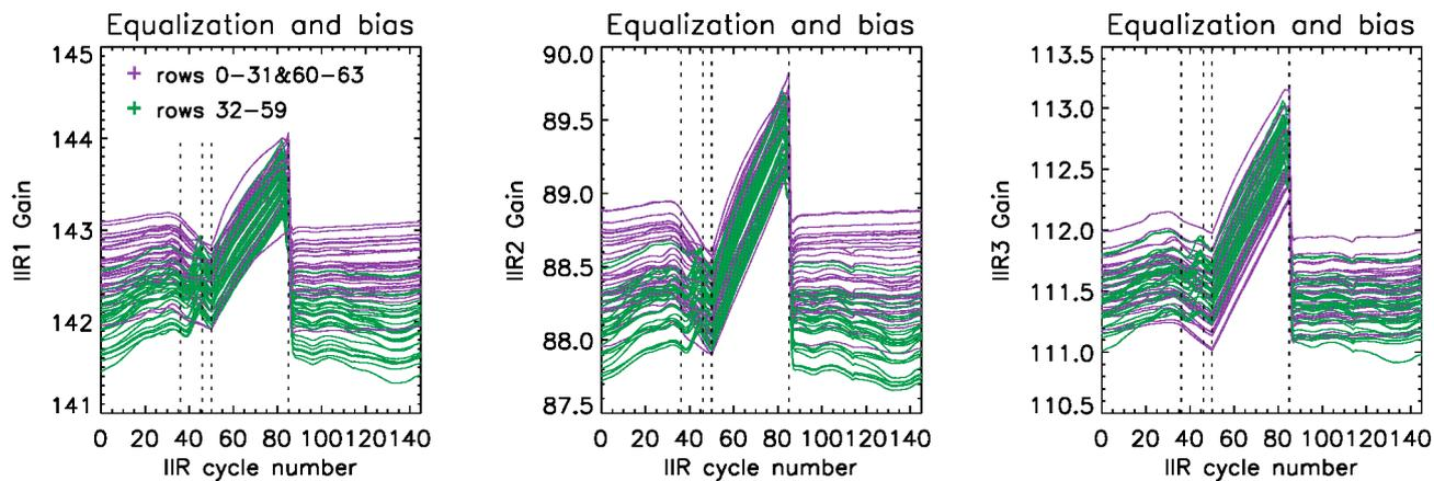
5 **Figure 8: Mean gains vs. IIR cycle number in June 2012 for each of the 64 rows in IIR1 (left), IIR2 (middle), and IIR3 (right) after equalization and bias corrections. Purple: sound rows; green: flawed rows.**
