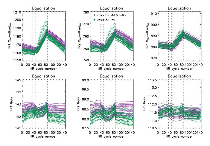
Figure 7: Mean digital counts in offset-corrected blackbody views after equalization correction (top) and resulting mean gains (bottom) vs. IIR cycle number in June 2012 for each of the 64 rows in IIR1 (left), IIR2 (middle), and IIR3 right). Purple: sound rows; green: flawed rows. The dashed green lines in the upper plots show the flawed rows before correction (cf Fig. 4).
