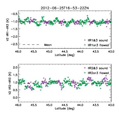
Figure 11: Version 2 IIR1-IIR3 (top) and IIR2-IIR3 (bottom) inter-channel BTDs in the same nighttime descending portion of the same orbit as in Figs. 1, 5, and 10. Purple: sound rows in both channels; green: flawed rows in at least one channel. Horizontal dashed line: mean value.
