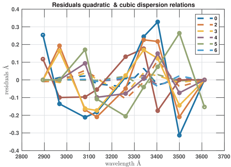
Figure 8. Residuals of the quadratic (filled circles, solid lines) and cubic (dashed lines) fits. The color indicates the six Brewer slits with the laser wavelengths in equally spaced grid every 5nm
