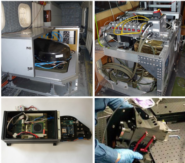
Figure 2. Overview of the four DOAS imaging instruments: APEX (top-left), AirMAP (top-right), SWING (bottom-left) and SBI (bottom-right).
