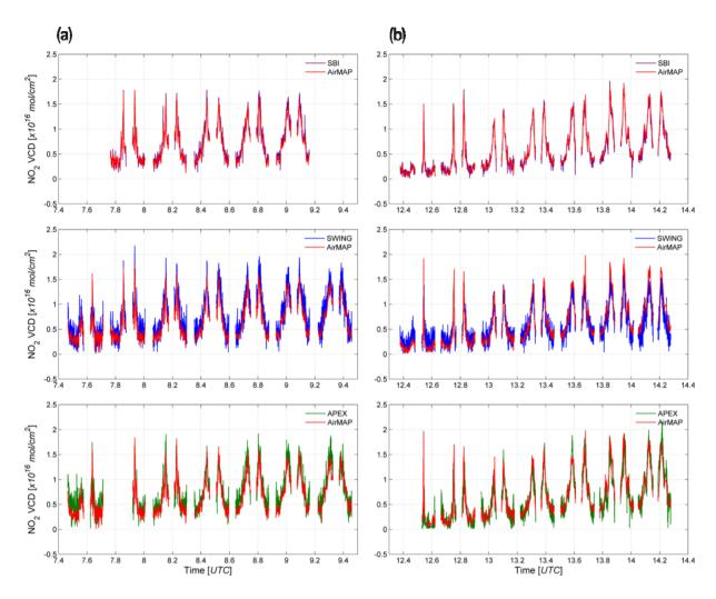
**Figure 18.** Co-located NO<sub>2</sub> VCDs retrieved from the harmonised maps for respectively **(a)** the morning and **(b)** afternoon flight on 21 April 2016. APEX VCDs are provided in green, AirMAP in red, SWING in blue and SBI in purple. The X-axis corresponds to the acquisition time, recorded by the Cessna 207T D-EAFU.
