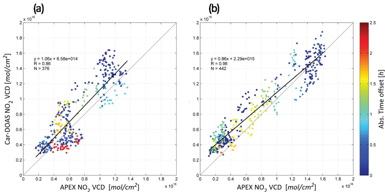
5 **Figure 15.** Scatter plots and linear regression analyses of the co-located  $\text{NO}_2$  VCDs, retrieved from APEX and car-DOAS for (a) the morning and (b) afternoon flight on 21 April 2016, respectively. Data points are colour-coded based on the absolute time offset between APEX and car-DOAS observations.
