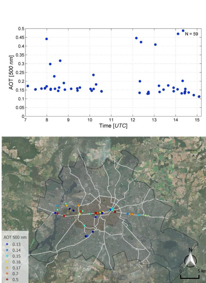
**Figure 5.** Time series (upper panel) and map (lower panel) of AOTs at 500 nm, measured with a Model 540 Microtops II handheld sun-photometer and operated from a car which was driving through the city of Berlin during the aircraft overpasses on 21 April 2016.
