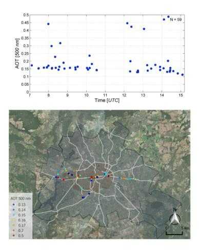
**Figure 5.** Time series (upper panel) and map (lower panel) of AOTs at 500 nm, measured with a Model 540 Microtops II handheld sunphotometer and operated from a car which was driving through the city of Berlin during the aircraft overpasses on 21 April 2016.
