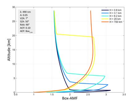
**Figure 8.** Height-dependent box-AMFs assessing the vertical sensitivity to NO<sub>2</sub>, illustrated for five different scenarios for the sensor altitude H, in km a.g.l.
