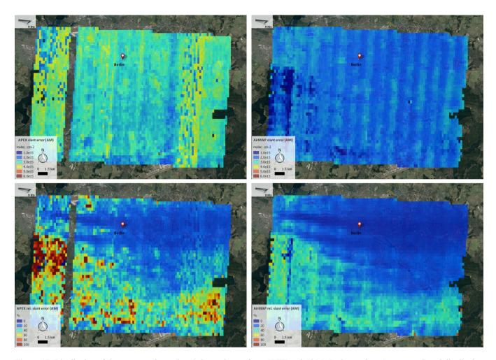
**Figure 17.** Distribution of the errors on the retrieved slant columns from APEX and AirMAP observations (upper panel) and distribution of the relative slant errors for APEX and AirMAP retrievals (lower panel) for the morning flight over Berlin on 21 April 2016 (Google, TerraMetrics).
