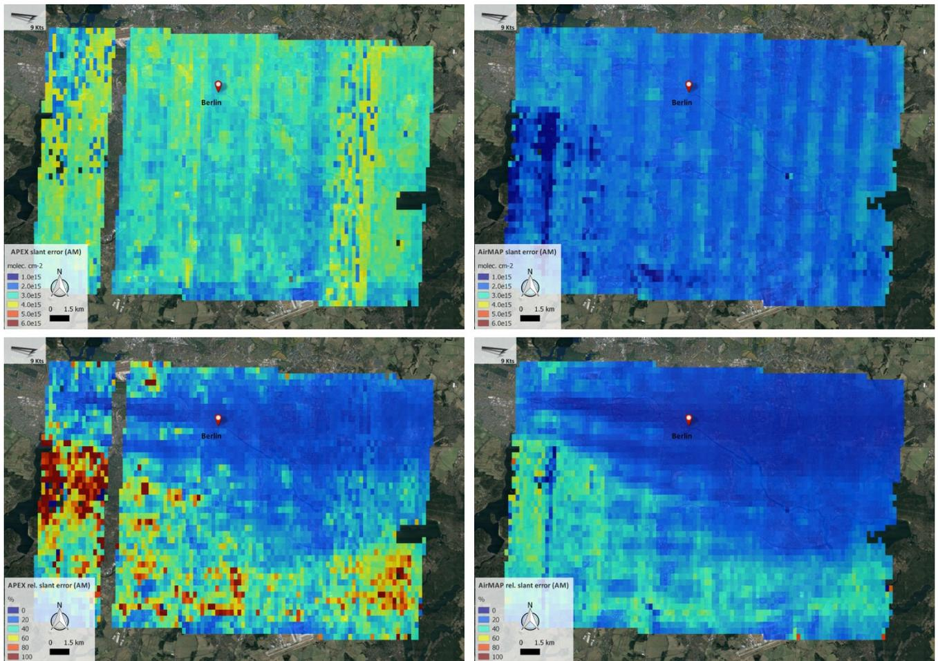
**Figure 17.** Distribution of the errors on the retrieved slant columns from APEX and AirMAP observations (upper panel) and distribution of the relative slant errors for APEX and AirMAP retrievals (lower panel) for the morning flight over Berlin on 21 April 2016 (Google, TerraMetrics).
