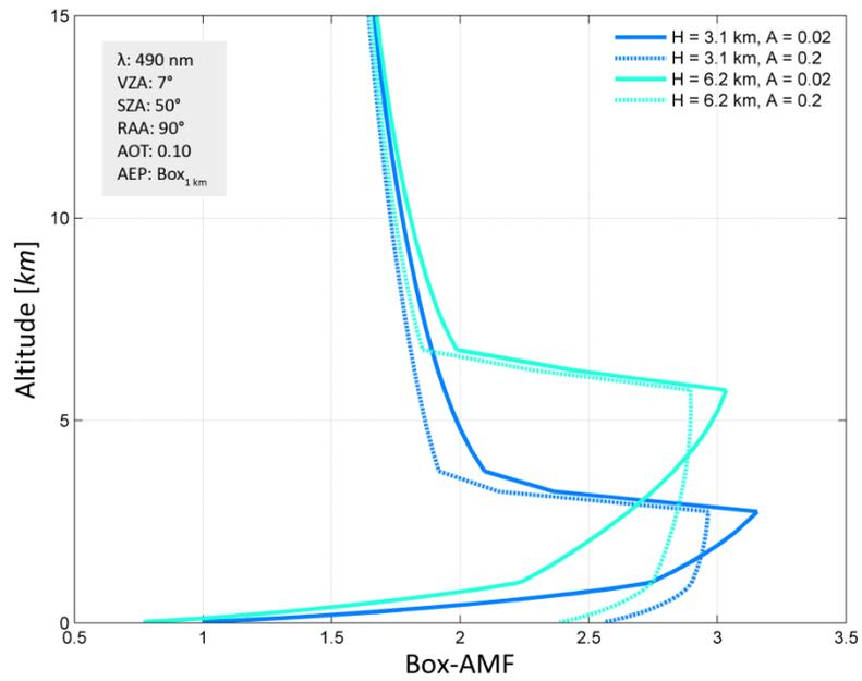
**Figure 9.** Height-dependent box-AMFs assessing the vertical sensitivity to NO<sub>2</sub>, illustrated for the aircraft altitude of the Cessna 207T D-EAFU (H = 3.1 km a.g.l.) and the Dornier DO-228 D-CFFU (H = 6.2 km a.g.l.), both for a low and high surface reflectance scenario.
