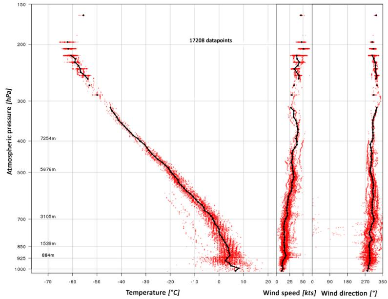
**Figure 13.** Temperature and wind profile on 21 April 2016 at 9 UTC, based on Mode-S-transponder data derived with an ADS-B-Receiver of ascending and descending aircraft in the vicinity of the two Berlin Airports (Bütow, 2016).
