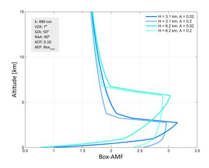
Figure 9. Height-dependent box-AMFs assessing the vertical sensitivity to  $NO_2$ , illustrated for the aircraft altitude of the Cessna 207T D-EAFU (H = 3.1 km a.g.l.) and the Dornier DO-228 D-CFFU (H = 6.2 km a.g.l.), both for a low and high surface reflectance scenario.
