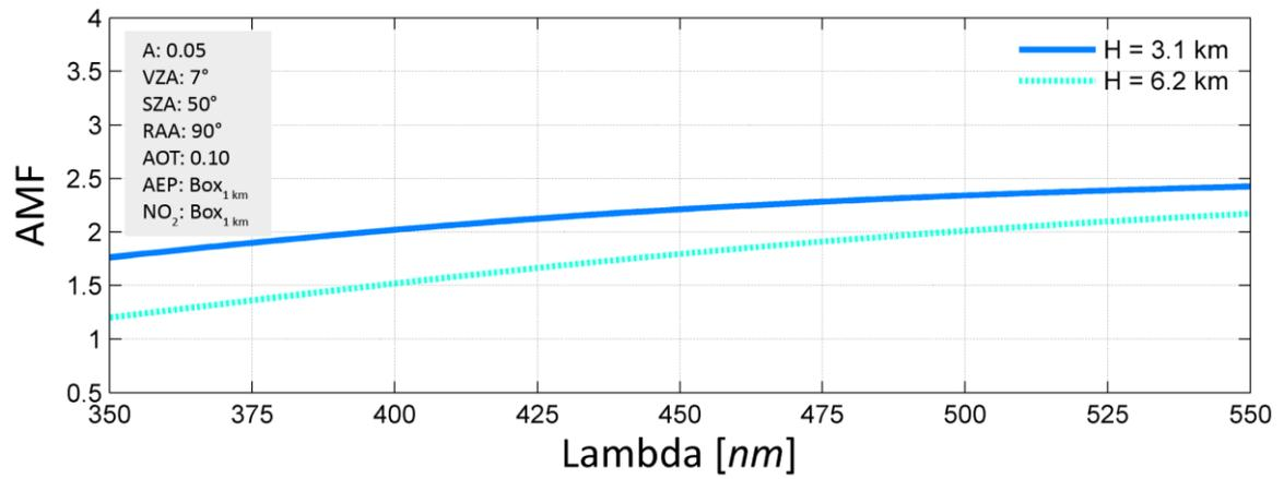
**Figure 10.** Dependence of the AMF on the surface reflectance and RTM computation wavelength ( $\lambda$ ) for the aircraft altitude of the Cessna 207T D-EAFU ( $H = 3.1$  km a.g.l.) and the Domier DO-228 D-CFFU ( $H = 6.2$  km a.g.l.).
