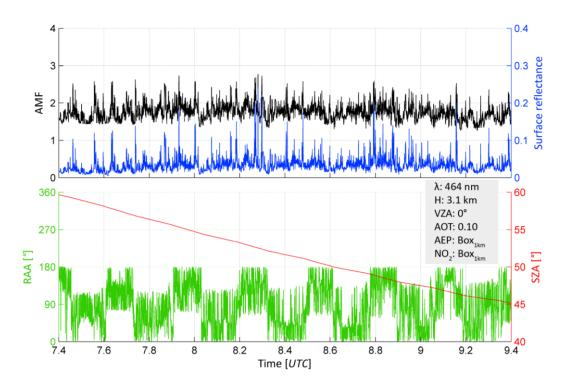
**Figure 6.** Time series of NO<sub>2</sub> AMFs for the morning flight on 21 April 2016, computed with DISORT based on the RTM parameters from the AirMAP instrument. The data is plotted for only the nadir observations in each across-track scanline.
