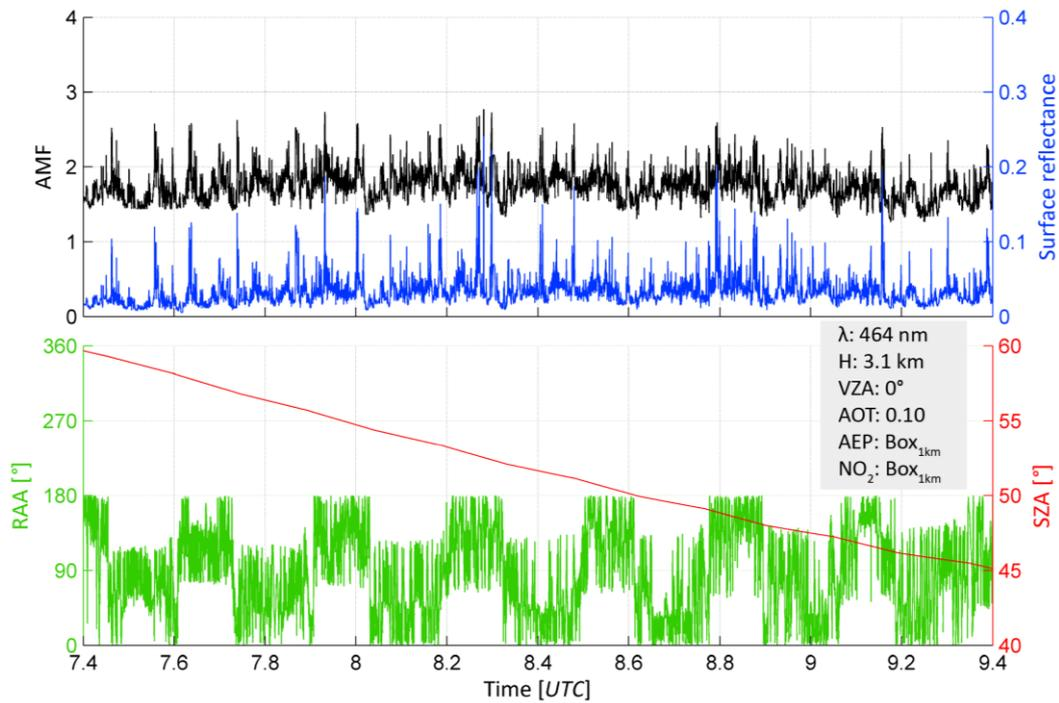
5 **Figure 6.** Time series of NO<sub>2</sub> AMFs for the morning flight on 21 April 2016, computed with DISORT based on the RTM parameters from the AirMAP instrument. The data is plotted for only the nadir observations in each across-track scanline.
