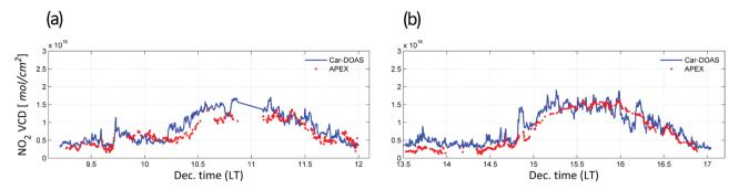
Figure 14. APEX and car-DOAS NO<sub>2</sub> VCD time series for (a) the morning and (b) afternoon flight on 21 April 2016, respectively.
