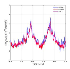
Figure 4. Zoom on the  $NO_2$  SCD time series of the morning flight over Berlin on 21 April 2016, between 08:21 and 08:36 UTC. The two  $NO_2$  peaks correspond to the crossings of the main plume with east-west orientation.
