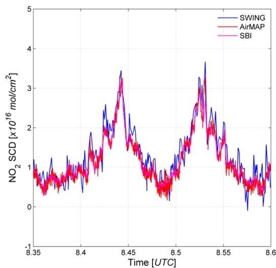
**Figure 4.** Zoom on the  $\text{NO}_2$  SCD time series of the morning flight over Berlin on 21 April 2016, between 08:21 and 08:36 UTC. The two  $\text{NO}_2$  peaks correspond to the crossings of the main plume with east-west orientation.
