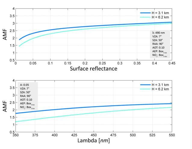
**Figure 10.** Dependence of the AMF on the surface reflectance and RTM computation wavelength ( $\lambda$ ) for the aircraft altitude of the Cessna 207T D-EAFU (H = 3.1 km a.g.l.) and the Dornier DO-228 D-CFFU (H = 6.2 km a.g.l.).
