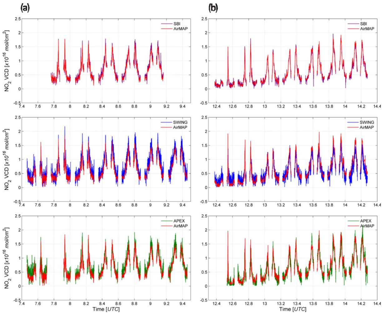
**Figure 18.** Co-located  $\text{NO}_2$  VCDs retrieved from the harmonised maps for respectively (a) the morning and (b) afternoon flight on 21 April 2016. APEX VCDs are provided in green, AirMAP in red, SWING in blue and SBI in purple. The X-axis corresponds to the acquisition time, recorded by the Cessna 207T D-EAFU.
