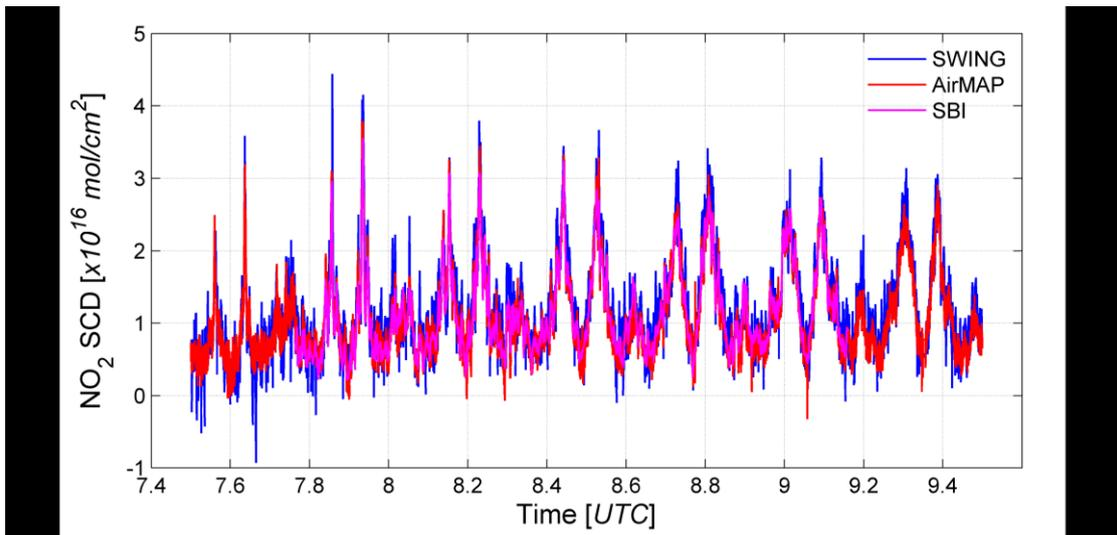
**Figure 3.** Time series of averaged  $\text{NO}_2$  near-nadir SCDs ( $> -4^\circ$  and  $< 4^\circ$  VZA), retrieved from AirMAP, SWING and SBI observations, during the morning flight over Berlin on 21 April 2016.
