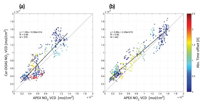
Figure 15. Scatter plots and linear regression analyses of the co-located NO<sub>2</sub> VCDs, retrieved from APEX and car-DOAS for (a) the morning and (b) afternoon flight on 21 April 2016, respectively. Data points are colour-coded based on the absolute time offset between APEX and car-DOAS observations.
