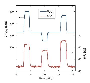
Figure 2: Example CRDS data feed for syringe samples. Reference air measurements (ca. 425 ppm  $x^{12}CO_2$  and -37 ‰  $\delta^{13}C-CO_2$ ) are interrupted by successive samples to form consistently identifiable peaks in the data.
