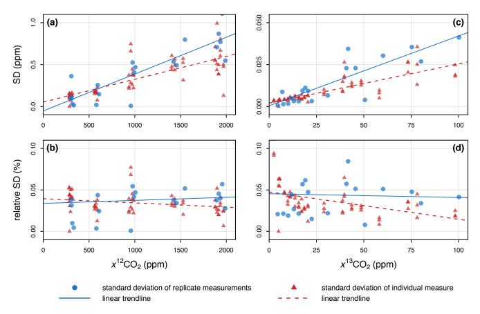
Figure 5: Precision in syringe sample data for  $x^{12}$ CO<sub>2</sub> (left: a, b) and  $x^{13}$ CO<sub>2</sub> (right: c, d) as quantified by standard deviations (top: a, c) and relative standard deviations (bottom: b, d) for individual measures (red) and replicate measurements (blue).
