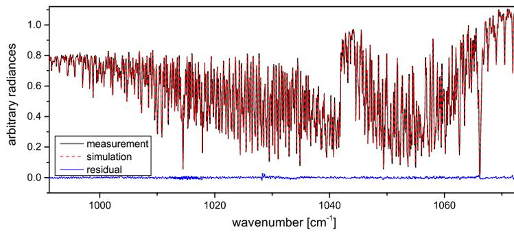
**Figure 4.** Same as Fig. 2 but for the spectral window used for the retrievals with the FTIR instrument at UNAM. Shown is an example for 22 March 2013, 17:57 UT; solar elevation:  $68.2^\circ$ ;  $O_3$  slant column: 285.4 DU.
