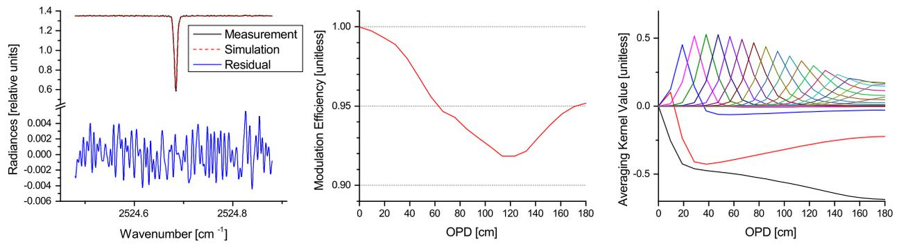
**Figure 11.** Typical ILS analysis for the IFS 120/5 at Alzomoni. Left panel: Example of cell spectrum and analysis; Middle panel: retrieved modulation efficiency; Right panel: averaging kernel for the modulation efficiency.
