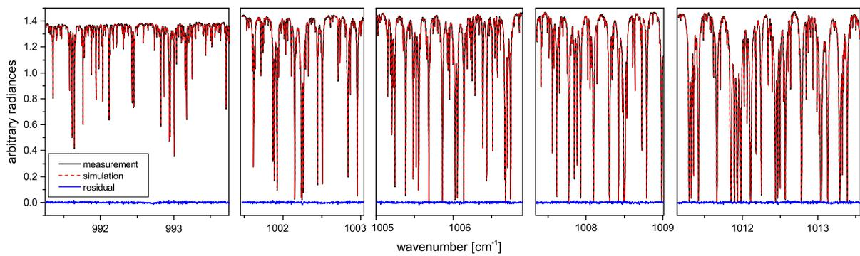
**Figure 2.** The spectral windows used for the retrievals with the NDACC FTIR instrument at Alzomoni. Shown is an example for a typical measurement (22 March 2013, 17:51 UT; solar elevation:  $67.9^\circ$ ;  $O_3$  slant column: 283 DU). Black line: measurement; red dashed line: simulation; blue line: residual (difference between measurement and simulation).
