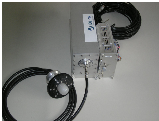
Figure 1. Basic components of a CCD array spectroradiometer system for airborne measurements. 2\pi receiver optics with optical fiber (black, front), spectrometer including monochromator and CCD array detector (middle), and cooling electronics (right).
