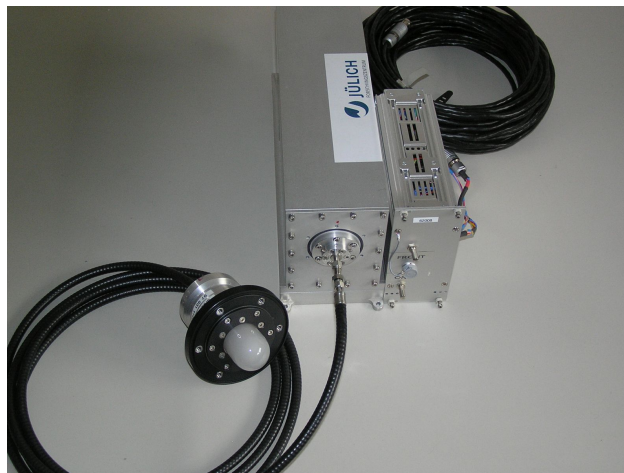
Figure 1. Basic components of a CCD array spectroradiometer system for airborne measurements. 2\pi receiver optics with optical fiber (black, front), spectrometer including monochromator and CCD array detector (middle), and cooling electronics (right).
