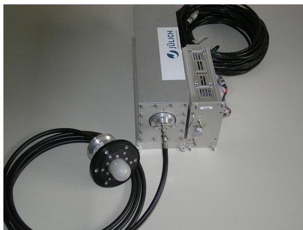
Figure 1. Basic components of a CCD array spectroradiometer system for airborne measurements. Receiver optics with optical fiber (black, front), spectrometer including monochromator and CCD array detector (middle), and cooling electronics (right).
