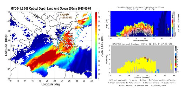
Figure 3: 3D profiling of the dust incursion on 1 Feb 2015: spatial extent provided by MODIS Level 2 (collection 6) AOD at 550nm (Left) together with CALIPSO profiles at 532nm of the extinction coefficient (Upper Right) and aerosol sub-typing (Lower Right) in the profile taken at 11:37 UTC (indicated by the distinct black-coloured track line in the left panel).
