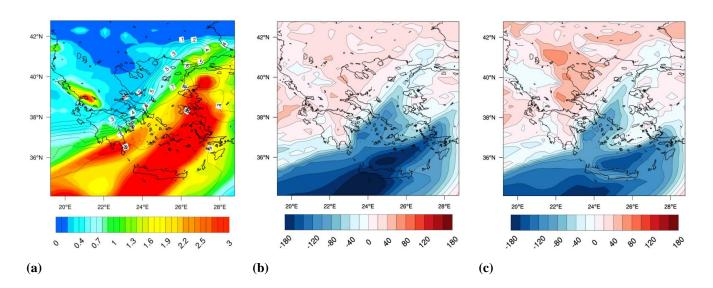
Figure 11: The spatial distribution of the: (a) total AOD (at 550nm). Iso-lines indicate the dust fraction of the total AOD model values. The map corresponds to 12:00 UTC, when maximum AOD  $\approx$  5.2. (b) dust plume effect on GHI and (c) DNI (in W/m<sup>2</sup>) at surface, averaged for the daytime hours of the extreme dust event of 1 Feb 2015 over Greece as predicted by COSMO-ART.
