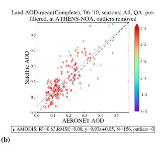
Figure 4: Scatter plots of satellite AOD (550nm) from MODIS/Aqua versus coincident AOD from AERONET for the five year period 2006-2010 with outliers removed. (a) shows the global record and (b) is for the ATHENS-NOA site. The colour bar describes the percentage frequency of AOD values occurrence (source of the plots: https://giovanni.gsfc.nasa.gov/mapss\_explorer).
