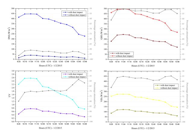
Figure 8: Temporal evolution of GHI, DNI, UV and VIS irradiances during the extreme dust event of 1 Feb 2015 at the Athens station. The modeled values (without dust impact) coincident with AERONET Cimel measurements (with dust impact) are shown together with the % attenuation due to impact of dust.
