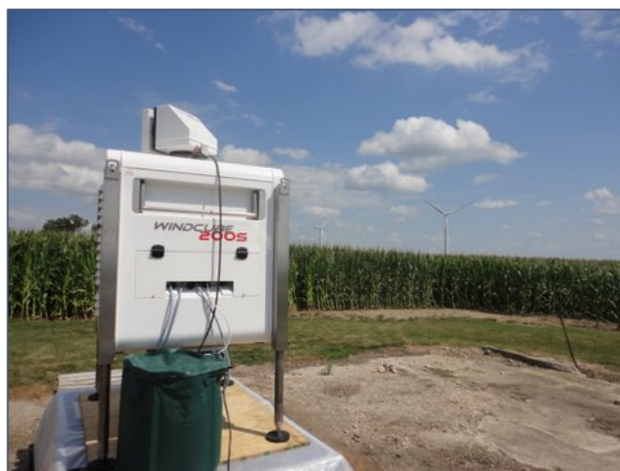
Figure 1: scanning lidar co-located with WC-3, looking to the southwest (photo courtesy Paul Quelet)
