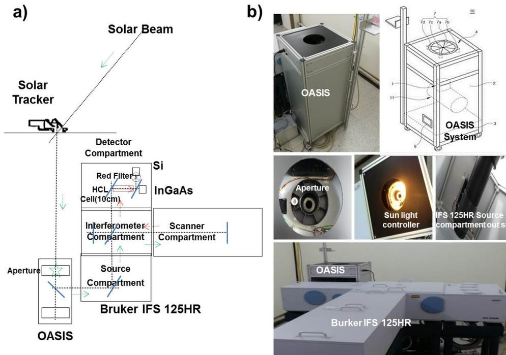
**Fig. 2.** Schematic views of the OASIS system.
