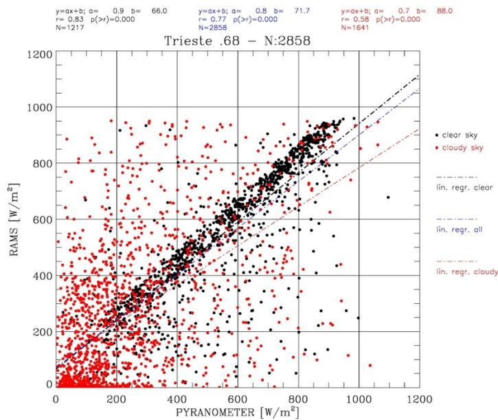
Figure 9 – Trieste (tri): a) scatter plot of the hourly GHI for the pyranometer (x-axis) and MSG (y-axis). The black dots are for clear sky conditions while the red dots are for both contaminated and overcast skies; b) as in a) for the RAMS one-day ahead hourly forecast. Regression lines are shown in their respective colours (blue is for all data, i.e. both clear and cloudy conditions).
