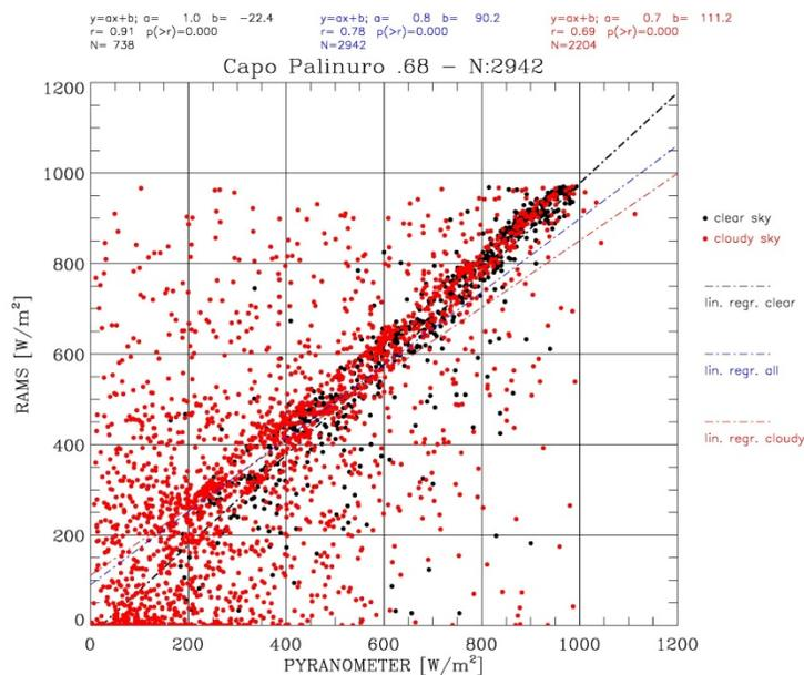
Figure 4 – Palinuro (pal): a) scatter plot of the hourly GHI for the pyranometer (x-axis) and MSG (y-axis). The black dots are for clear sky conditions while the red dots are for both contaminated and overcast skies; b) as in a) for the RAMS one-day ahead hourly forecast. Regression lines are shown in their respective colours (blue is for all data, i.e. both clear and cloudy conditions).
