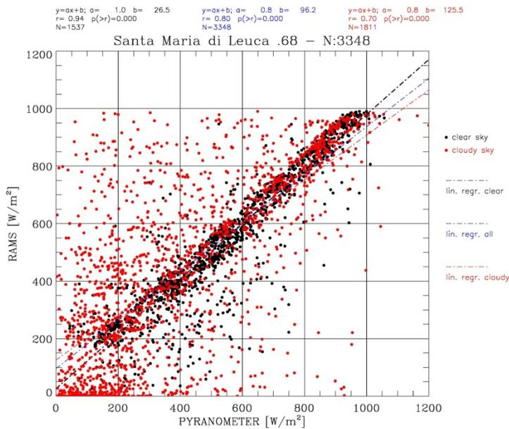
Figure 3 – Santa Maria di Leuca (sml): a) scatter plot of the hourly GHI for the pyranometer (x-axis) and MSG (y-axis). The black dots are for clear sky conditions while the red dots are for both contaminated and overcast skies; b) as in a) for the RAMS one-day ahead hourly forecast. Regression lines are shown in their respective colours (blue is for all data, i.e. both clear and cloudy conditions).
