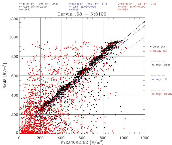
Figure 8 – Cervia (cer): a) scatter plot of the hourly GHI for the pyranometer (x-axis) and MSG (y-axis). The black dots are for clear sky conditions while the red dots are for both contaminated and overcast skies; b) as in a) for the RAMS one-day ahead hourly forecast. Regression lines are shown in their respective colours (blue is for all data, i.e. both clear and cloudy conditions).
