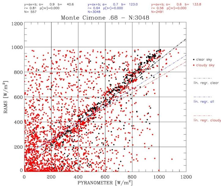
Figure 10 – Monte Cimone (cim): a) scatter plot of the hourly GHI for the pyranometer (x-axis) and MSG (y-axis). The black dots are for clear sky conditions while the red dots are for both contaminated and overcast skies; b) as in a) for the RAMS one-day ahead hourly forecast. Regression lines are shown in their respective colours (blue is for all data, i.e. both clear and cloudy conditions).
