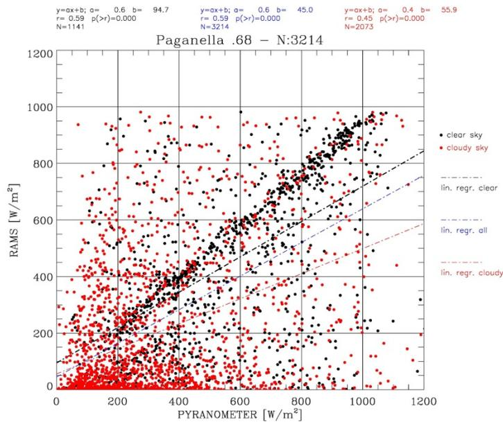
Figure 11 – Paganella (pag): a) scatter plot of the hourly GHI for the pyranometer (x-axis) and MSG (y-axis). The black dots are for clear sky conditions while the red dots are for both contaminated and overcast skies; b) as in a) for the RAMS one-day ahead hourly forecast. Regression lines are shown in their respective colours (blue is for all data, i.e. both clear and cloudy conditions).
