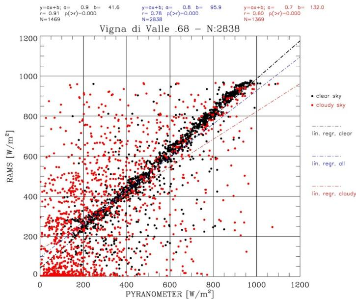
Figure 6 – Vigna di Valle (vdy): a) scatter plot of the hourly GHI for the pyranometer (x-axis) and MSG (y-axis). The black dots are for clear sky conditions while the red dots are for both contaminated and overcast skies; b) as in a) for the RAMS one-day ahead hourly forecast. Regression lines are shown in their respective colours (blue is for all data, i.e. both clear and cloudy conditions).
