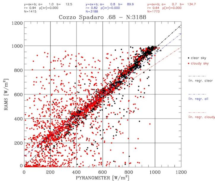
Figure 2 – Cozzo Spadaro (csp): a) scatter plot of the hourly GHI for the pyranometer (x-axis) and MSG (y-axis). The black dots are for clear sky conditions while the red dots are for both contaminated and overcast skies; b) as in a) for the RAMS one-day ahead hourly forecast. Regression lines are shown in their respective colours (blue is for all data, i.e. both clear and cloudy conditions).
