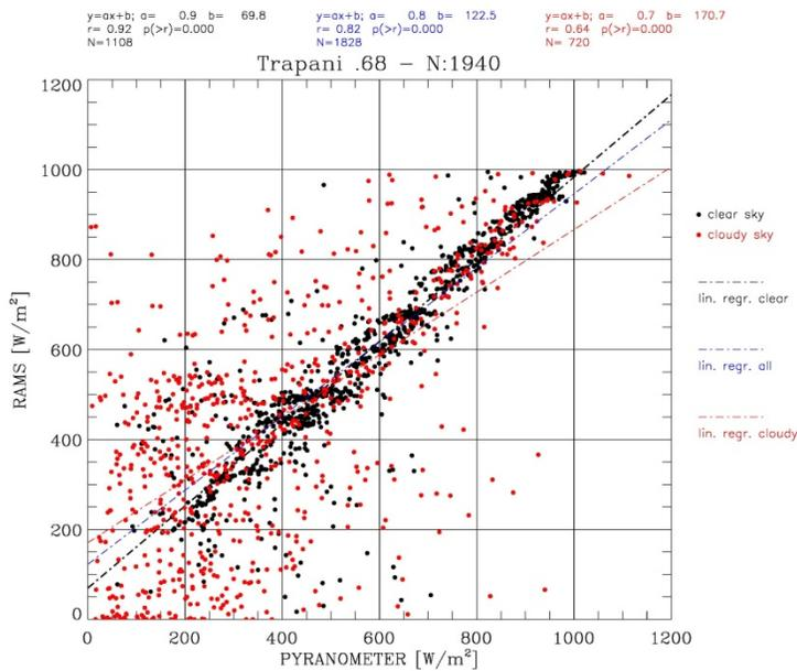
Figure 1 – Trapani (tra): a) scatter plot of the hourly GHI for the pyranometer (x-axis) and MSG (y-axis). The black dots are for clear sky conditions while the red dots are for both contaminated and overcast skies; b) as in a) for the RAMS one-day ahead hourly forecast. Regression lines are shown in their respective colours (blue is for all data, i.e. both clear and cloudy conditions).
