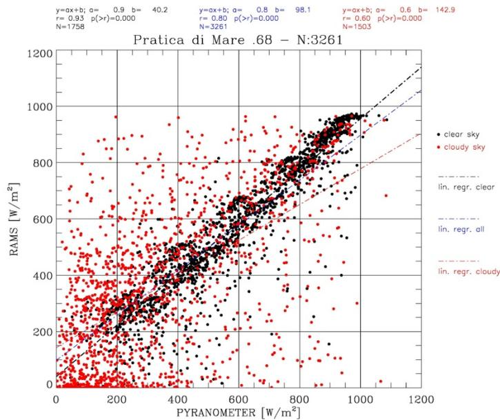
Figure 5 – Pratica di Mare (pdm): a) scatter plot of the hourly GHI for the pyranometer (x-axis) and MSG (y-axis). The black dots are for clear sky conditions while the red dots are for both contaminated and overcast skies; b) as in a) for the RAMS one-day ahead hourly forecast. Regression lines are shown in their respective colours (blue is for all data, i.e. both clear and cloudy conditions).
