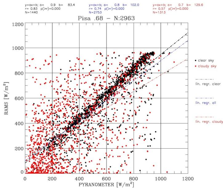
Figure 7 – Pisa (pis): a) scatter plot of the hourly GHI for the pyranometer (x-axis) and MSG (y-axis). The black dots are for clear sky conditions while the red dots are for both contaminated and overcast skies; b) as in a) for the RAMS one-day ahead hourly forecast. Regression lines are shown in their respective colours (blue is for all data, i.e. both clear and cloudy conditions).
