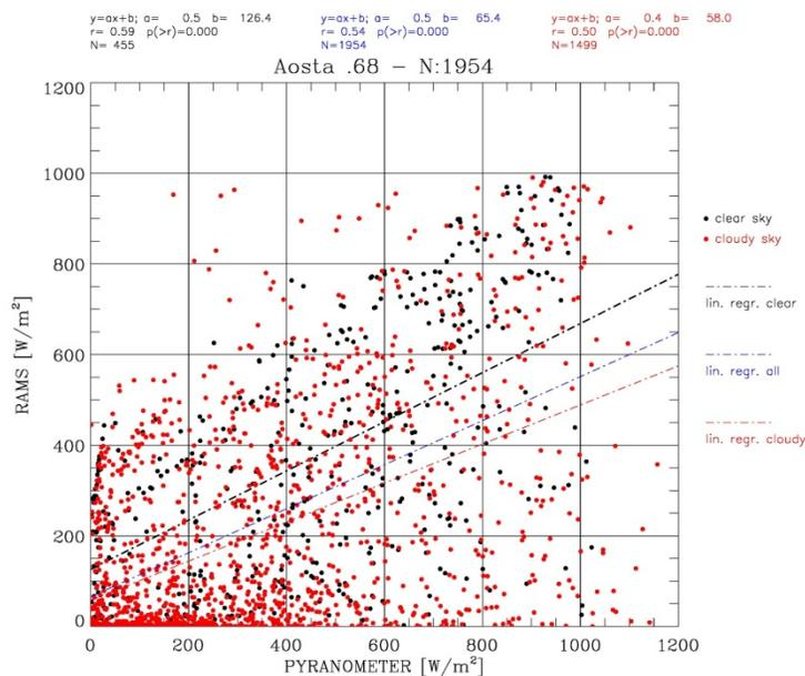
Figure 12 – Aosta (aos): a) scatter plot of the hourly GHI for the pyranometer (x-axis) and MSG (y-axis). The black dots are for clear sky conditions while the red dots are for both contaminated and overcast skies; b) as in a) for the RAMS one-day ahead hourly forecast. Regression lines are shown in their respective colours (blue is for all data, i.e. both clear and cloudy conditions).
