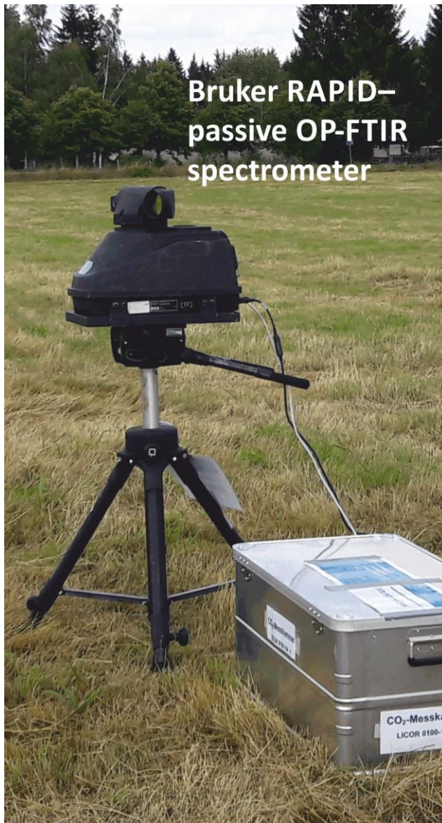
Figure 3. OP-FTIR spectrometer used for SOP at Grillenburg site. Left: passive Bruker RAPID, right: active Bruker EM27 detector unit applied in bistatic mode with a separate IR source (not in figure).
