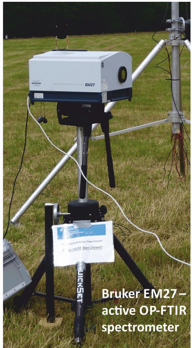
Figure 3. OP-FTIR spectrometer used for SOP at Grillenburg site. Left: passive Bruker RAPID, right: active Bruker EM27 detector unit applied in bistatic mode with a separate IR source (not in figure).
