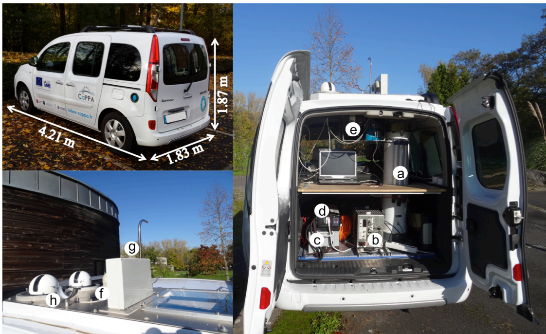
Figure 1. Mobile system and equipment: (a) LiDAR transmitter-receiver optical head, (b) LiDAR control and acquisition unit, (c) battery, (d) sine-wave inverter charger, (e) aerosol spectrometer, (f) meteorological probe, (g) isokinetic sampling probe and (h) PLASMA sun photometers.
