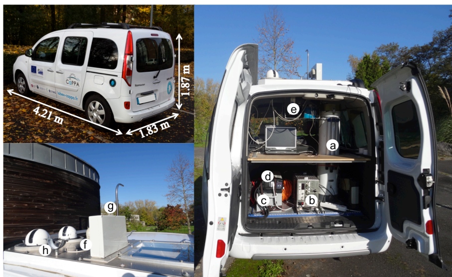
5 Figure 1. Mobile system and equipment: (a) LiDAR transmitter-receiver optical head, (b) LiDAR control and acquisition unit, (c) battery, (d) sine-wave inverter charger, (e) aerosol spectrometer, (f) meteorological probe, (g) isokinetic sampling probe and (h) PLASMA sun photometers.
