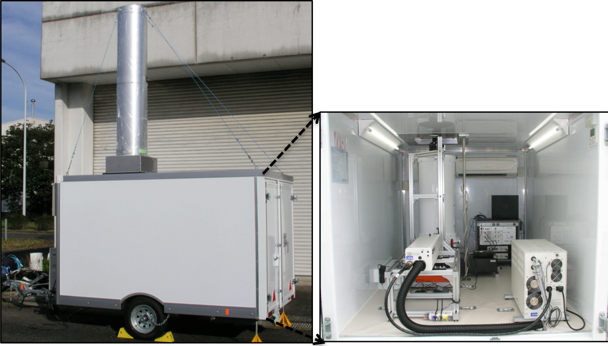
Figure 3. Photographs of the mobile RL-MRL trailer (left) and its interior (right).
