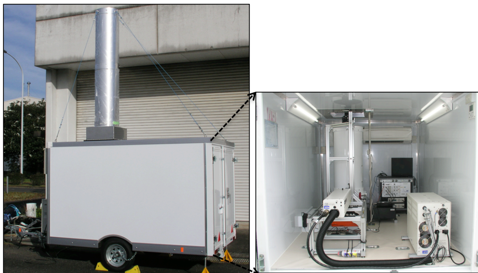
Figure 2. Layout of the mobile Raman lidar system in its trailer. Dimensions are in millimeters.
