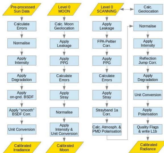
**Figure 3.** Processing flow indicating the order of steps for calculating the calibrated level 1 science data, i.e. irradiance (left column), moon radiance (middle column), and earthshine radiance (right columns). See text for detailed explanations.
