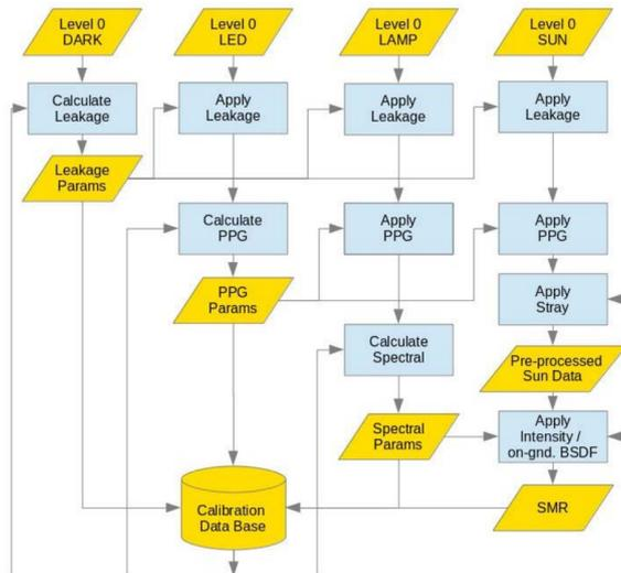
**Figure 2.** Processing flow for calculating the in-flight calibration parameters from the dark signal measurements (DARK), the internal LED measurements (LED), the spectral lamp measurements (LAMP), and the solar measurements (SUN). The calibration parameters as well as the Sun Mean Reference (SMR) spectrum are stored in the calibration data base.
