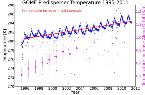
**Figure 10.** Temperature measured at the pre-disperser prism as a function of time from 1995 to 2011 (blue) and linear fit (red). The temperature increase is about  $2.5 \text{ K decade}^{-1}$ . Magenta dots denote the increase of the pre-disperser temperature along one orbit in Kelvin hour $^{-1}$  (right y-axis) for the years 1995 to 2003. Analysis of later years is not possible due to the tape recorder failure (incomplete orbits).
