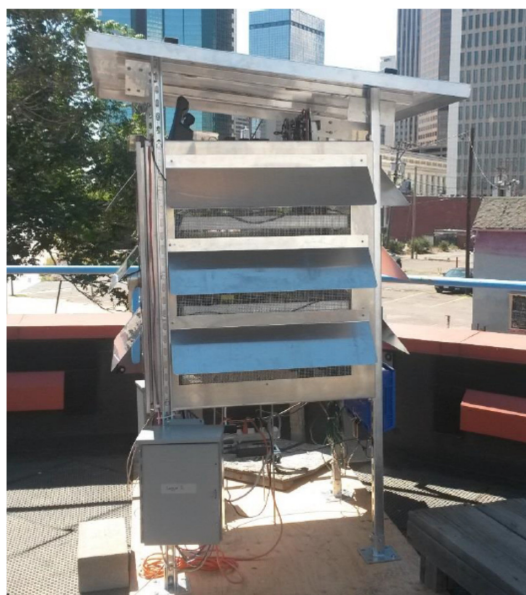
139 Figure 1 Sensor deployment shelter
