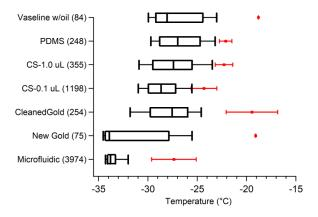
Figure 11. Summary of pure water droplet freezing spectra for different substrates tested. Boxes show the 25% and 75% frozen quartiles and the median, N<sub>50</sub>, is indicated by the line inside each box. Red markers are the temperatures of the first onset freezing droplets with error bars showing variability between different replicate
