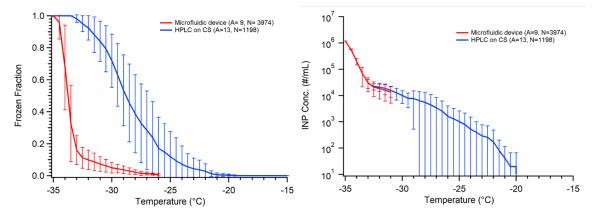
535 Figure 10. Comparison of pure water droplet freezing in our new microfluidic chip (red) versus using a silanized cover slip (CS) (blue), following Figure 5. Droplets in the microfluidic chip are 6 nL in volume and droplets on the CS are 0.1 μL. Error bars show variability of droplet freezing between different replicate arrays. The parentheses next to each legend entry contains the number of arrays of droplets (A) and the total number of droplets across all arrays (N).
