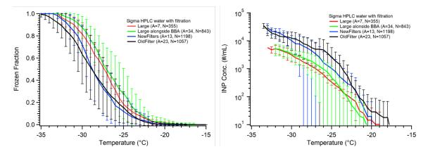
Figure 5. Droplet freezing temperature spectra (left) and apparent ice nuclei concentration, c<sub>IN</sub>, (right) for pure water droplet freezing measurements on a hydrophobic cover slip. In all experiments HPLC water that was filtered using an Anotop 0.02 um syringe filter was used. Each data series has been binned into 0.5 °C temperature
