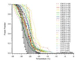
335 Figure 4. A series of tests on MilliQ generated water droplets to determine contamination sources. Droplets displayed inexplicably high freezing temperatures compared to filtered HPLC water at the time (solid brown with error bars). Temperatures for N<sub>50</sub> ranged from -20 °C to -29 °C from day to day. Error bars indicate standard deviation of data for the filtered HPLC water.
