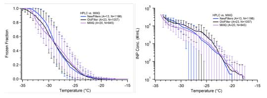
Figure 3. Comparison of pure water freezing using filtered MilliQ produced water and filtered purchased HPLC
