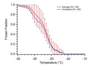
**Figure 1.** Comparison of averaging data from droplet freezing experiments on 120 total droplets measured using three replicate arrays of 40 droplets each (red with error bars) versus combining those 120 droplets into one single hypothetical array of droplets (blue). The standard deviation from the average of the three replicate arrays is shown by the vertical error bars.
