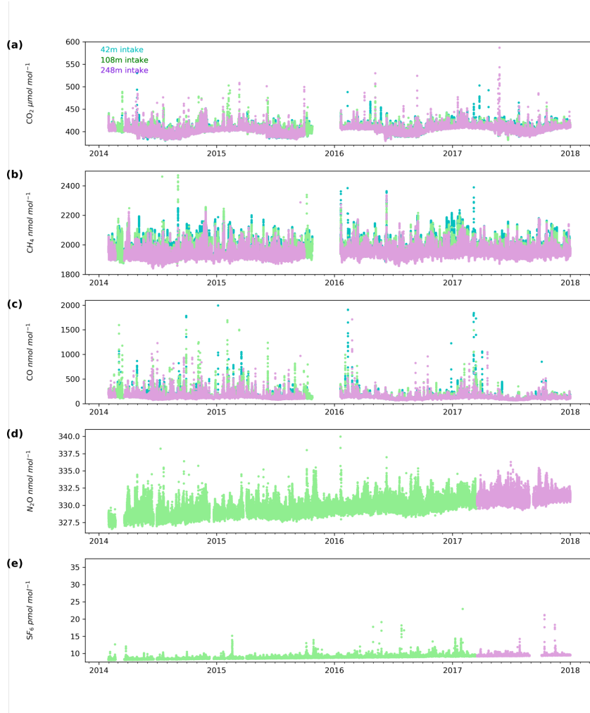
Figure 4: Minute mean (a) CO 2 , (b) CH 4 and (c) CO and 10 minute discrete (d) N 2 O and (e) SF 6 observations at the Bilsdale site for the 42 m (blue), 108 m (green) and 248 m (purple) intake heights.
