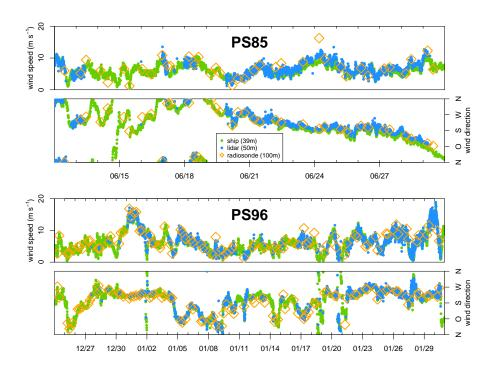
**Figure 7.** Comparison of wind speed (ff) and wind direction (dd) between lidar at 50 m height (blue) and ship anemometer (green) for PS85 (top) and PS96 (bottom). Radiosonde winds at 100 m are marked (orange diamond) for reference. Only scans with an elevation of 75° were used.
