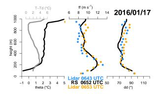
Figure 11. As Figure 9 but for the LLJ around 0700 UTC 17 January 2016 (PS96). A SNR threshold of -26 dB was used.
