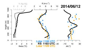
**Figure 9.** Vertical profiles of potential temperature (theta), dew-point spread (T-Td), wind speed (ff) and direction (dd) of radiosondes vs lidar wind speed and direction for around 1100 UTC 12 June 2016. A SNR threshold of -23 dB was used.
