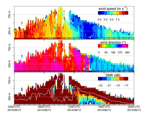
**Figure 8.** Lidar wind speed (top) and direction (middle) for -23 dB SNR threshold for the 12 June 2014 (location see PS85 in Fig. 1). Colors below the black line (40 m) show the wind measurements of RV *Polarstern* (anemometer). The bottom plot presents the SNR thresholds that would allow for a wind calculation. Grey line is the cloud base from ceilometer measurements of RV *Polarstern*.
