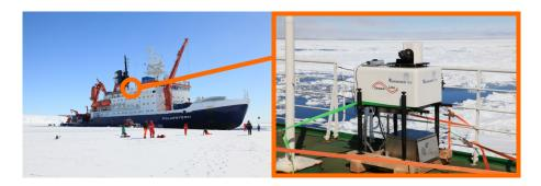
Figure 2. Position of the lidar on the RV Polarstern
