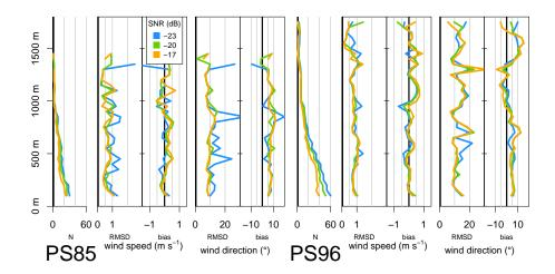
**Figure 6.** RMSD, bias and number of used radio soundings (N) by height of wind speed and direction for PS85 (left) and PS96 (right). Different colors show different SNR thresholds (-23 dB blue, -20 dB green, -17 dB orange). Only scans with an elevation of 75° were used.
