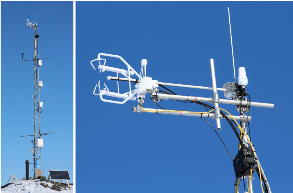
Figure 2. Photograph of the tower (left) and the flux instruments mounted at the top of the tower (right).
