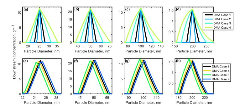
**Figure S1** (a-d) Downstream aerosols concentrations, cm<sup>-3</sup>, for DMA Cases 1-4, with sheath and excess air flow 3 L min<sup>-1</sup>, and aerosol and sample flow of 0.06-0.90 L min<sup>-1</sup>. (e-h) Downstream concentrations for DMA Cases 1 and 5-7, with sheath air flow 3.0 L min<sup>-1</sup>, sample flow 0.30 L min<sup>-1</sup>, and excess air flow 2.94-3.06 L/min.
