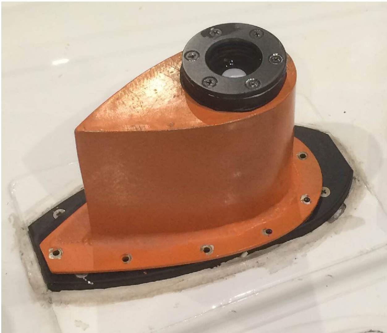
Figure 1. The zenith mounted OrangeCan on top of the NASA LaRC UC-12B aircraft. The remote cosine receptor RCR optic was mounted inside directly under a BK7 optical window to characterize sky conditions during flight.
