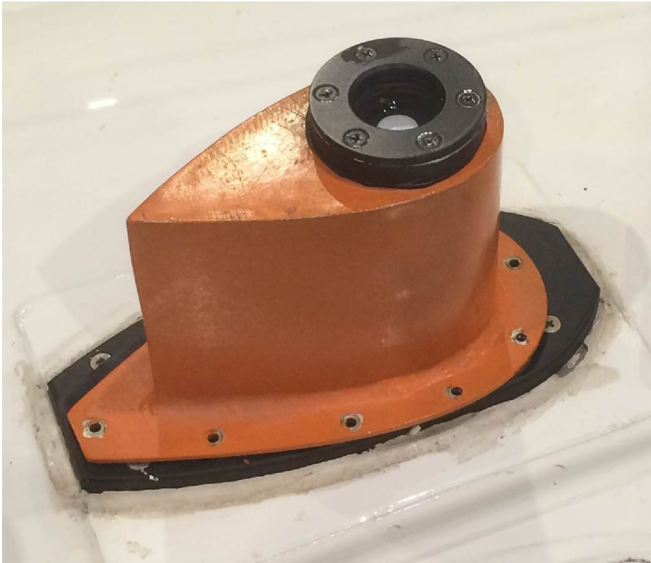
Figure 1. The zenith mounted OrangeCan on top of the UC-12B aircraft. The remote cosine receptor optic was mounted inside directly under a BK7 optical window to characterize sky conditions during flight.
