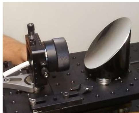
Figure 1: Fiber-coupled OAP configuration.
