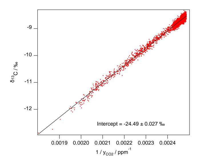
Figure 4. Keeling plot of data shown in Figure 2.
