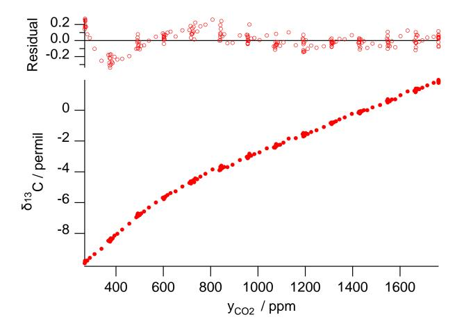
Figure 1. Example of  $\delta^{13}$ C dependence on CO<sub>2</sub> mole fraction for a Spectronus FTIR analyser. The measured data are fitted with a function of form of Eq. (15) with fitted parameters  $\beta = -1227 \%$  ppm and  $\gamma = 0.0054 \%$  ppm<sup>-1</sup>.
