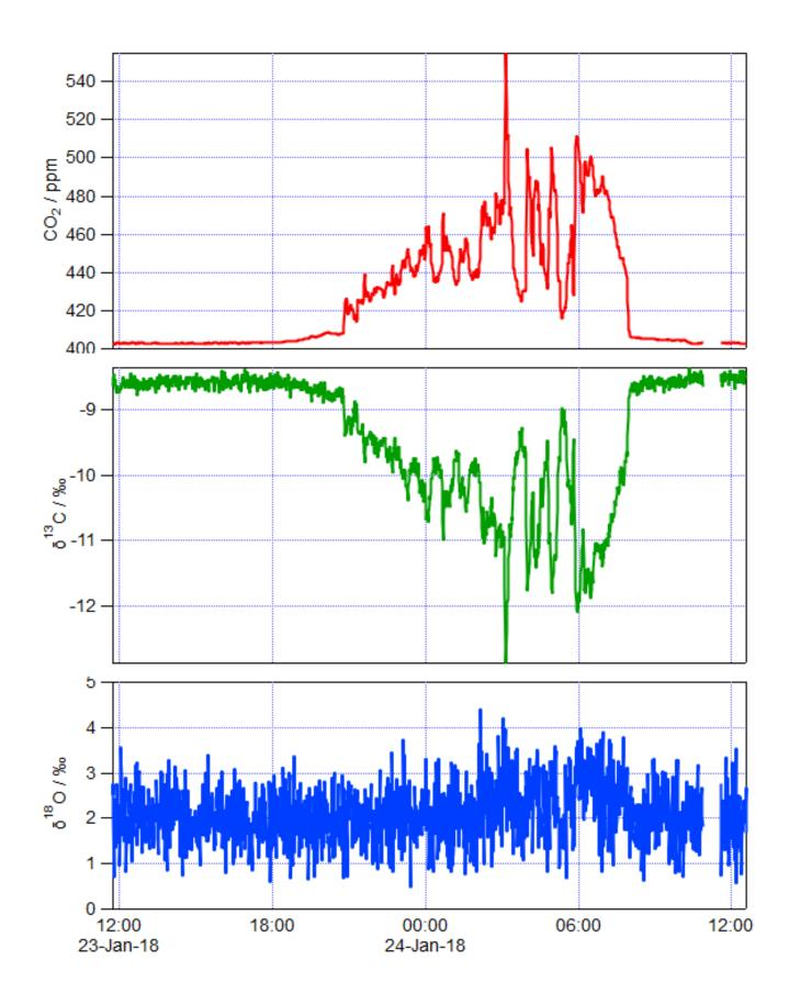
Figure 3. Calibrated total CO<sub>2</sub>,  $\delta^{13}$ C and  $\delta^{18}$ O of sampled air on 23-24 Jan 2018 at a rural site in SE Australia. Air was sampled continuously, the displayed data are 1 minute averages.
