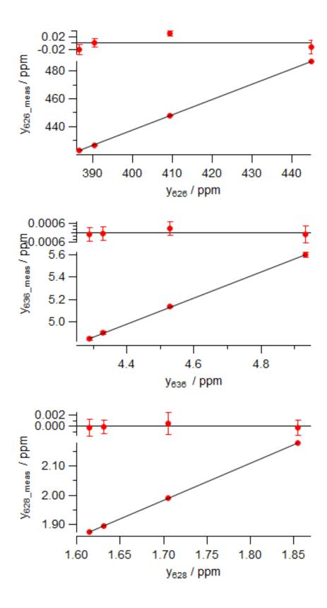
Figure 2. Calibration plots for three CO<sub>2</sub> isotopologues.
