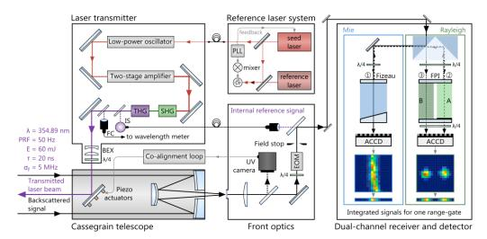
**Figure 1.** Schematic of the ALADIN Airborne Demonstrator (A2D) wind lidar instrument consisting of an injection-seeded, frequency-tripled laser transmitter, a Cassegrain telescope, front optics and a dual-channel receiver. PLL: phase locked loop, SHG: second harmonic generator, THG: third harmonic generator, IS: integrating sphere, FC: fiber coupler, BEX: beam expander, EOM: electro-optic modulator, FPI: Fabry-Pérot interferometer, ACCD: accumulation charge-coupled device.
