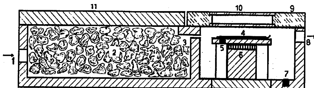
Figure S6. 1: air inlet; 2: minced ice; 3: slit and air temperature thermocouple; 4: filter; 5: filter temperature thermocouple; 6: Peltier cooling device; 7: thermocouple; 8: air outlet; 9: plexiglass cover; 10: observation slit; 11: aluminium plate.
