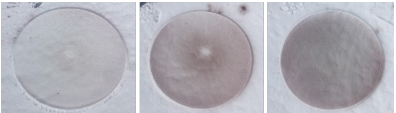
Figure 4: Images of three hematite depositions allow for visual inspection of the deposition uniformity . The left and center panels represent a previous apparatus design which featured a fan mounted inside the deposition chamber, which created less-uniform depositions . The right panel represents a hematite deposition using the final configuration of the apparatus .
