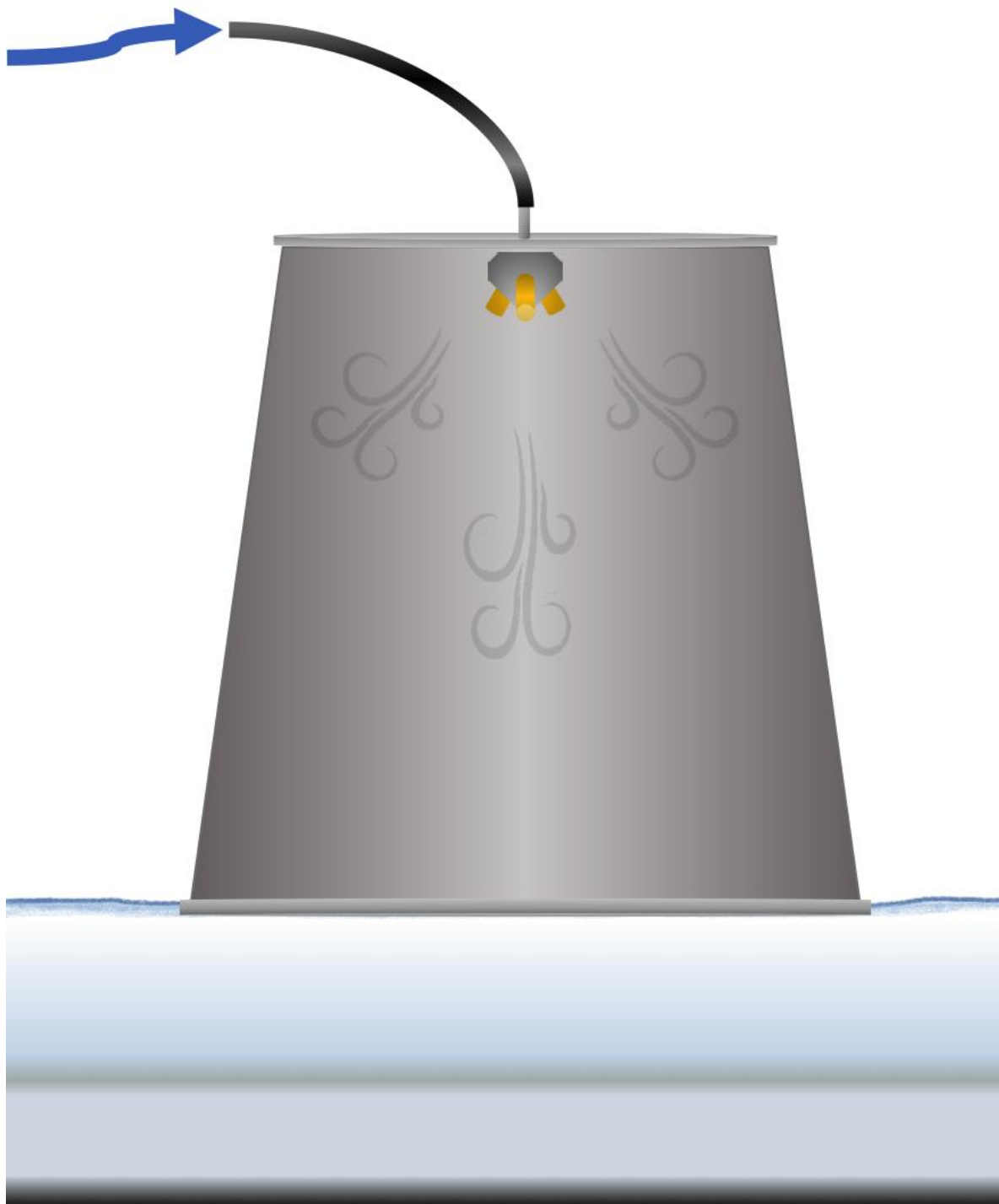
Figure 2: The deposition chamber for all aerosol types consists of a near cylindrical volume with aerosols pumped into the inlet at the top of the chamber from the production or entrainment chamber.
