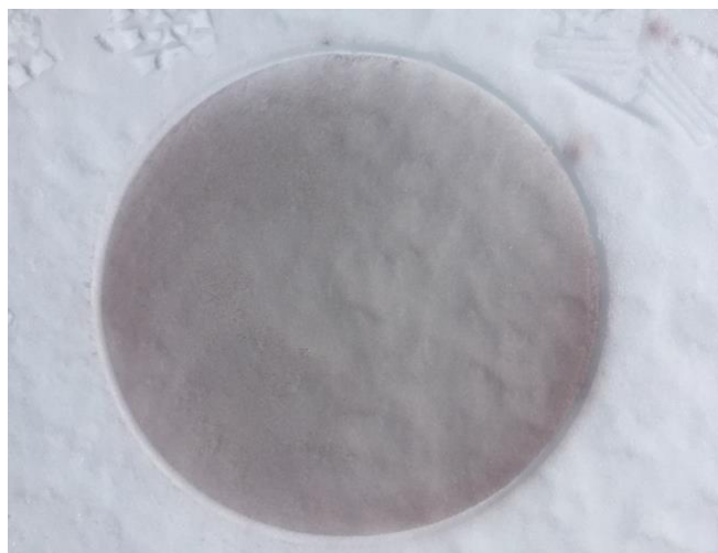
Figure 7: Image and HCRF spectra for a hematite deposition and adjacent natural snow in May of 2016 at the CUES research site. This hematite deposition drastically reduced the high natural snow reflectivity in the ultraviolet and short-wavelength visible (< 600 nm) spectral regions.
