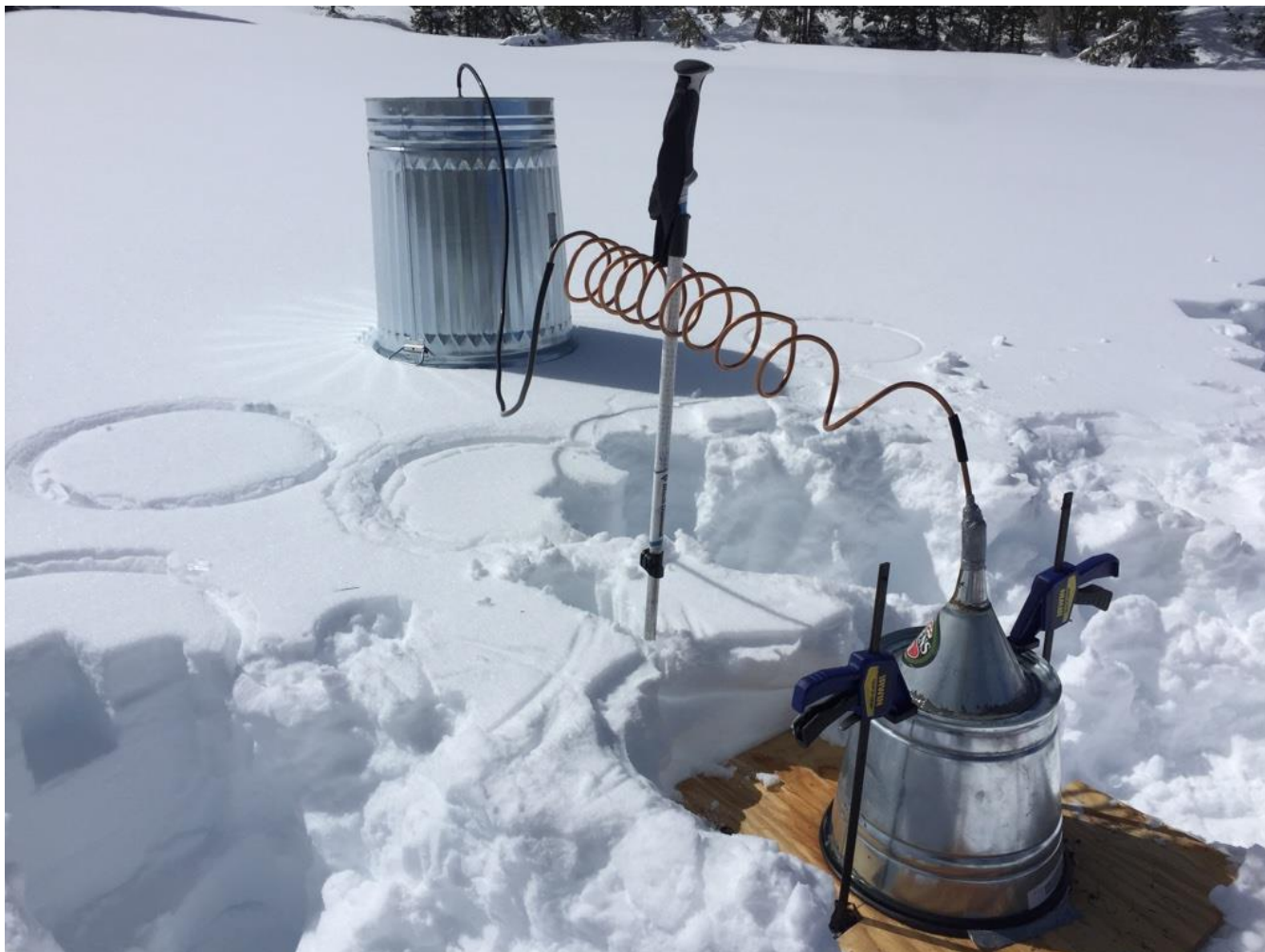
Figure 3: Use of the apparatus at the Tamarack Lake site for depositing BC aerosol.
