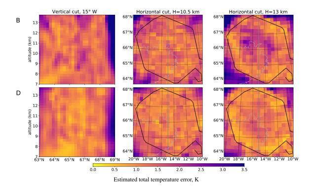
**Figure 6.** Panels show the Monte Carlo estimate of the total temperature error for retrievals B and D. In columns 2 and 3: black line – flight path, thick grey line – position of cut shown in the first column, thin grey line – topography.
