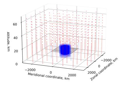
**Figure 2.** Grid for retrieval D. Radial distance is defined as distance to the vertical line at the centre of the hexagonal flight path ( $66^{\circ}$ N,  $15^{\circ}$ W). Points within the inner core (1000 km × 1000 km × 20 km) are shown in blue, other points – in red, shaded rectangle shows the position of horizontal cut in Figure 1b.
