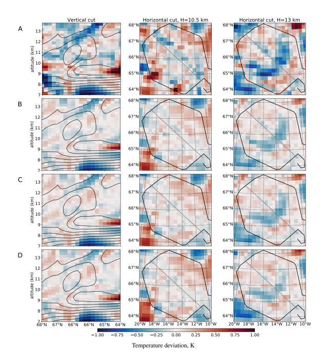
**Figure 4.** Panels show difference between retrieved temperature and true temperature of the simulated atmosphere. Rows A-D show results of respective retrievals. In the first column, black lines represent contours of a priori temperature value. In columns 2 and 3: black line – flight path, thick grey line – position of cut shown in the first column, thin grey line – topography (Icelandic coastline visible).
