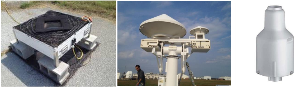
Figure 5: Instruments used in this study (from left to right): 2DVD (SN37), D3R (Dual-wavelength Dual-polarized Doppler Radar), and OTT Pluvio 2 400 precipitation gauge.
