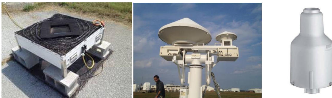
Figure 5: Instruments used in this study (from left to right): 2DVD (SN37), D3R (Dual-polarized Doppler Radar), and OTT Pluvio 2 400 precipitation gauge.
