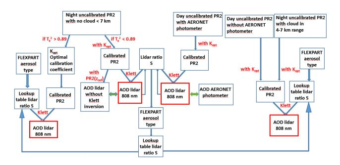
**Figure 4.** Flowchart of the lidar range-corrected signal (PR2) processing to derive the 800 nm aerosol optical depth (AOD) up to the reference altitude ( $z_{ref}$ ). Four different calibration and AOD calculation are used according to the measurement conditions. Iteration between the AOD calculation and the lidar ratio value is only possible when the AOD can be compared to an external AOD reference (green two-sided arrows).
