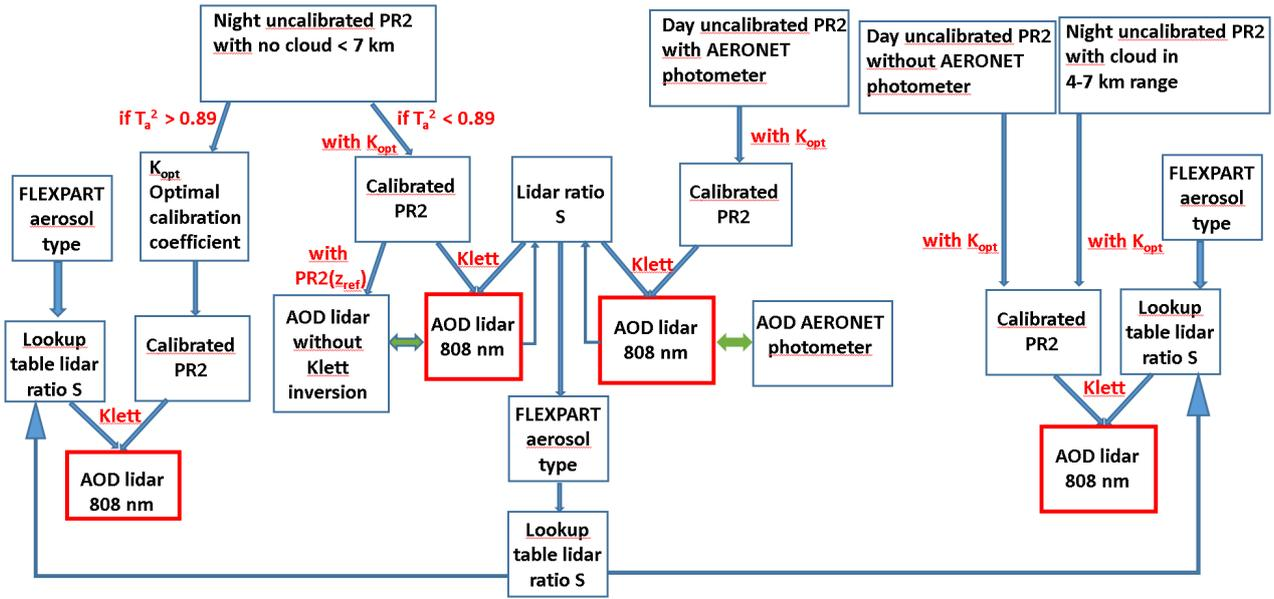
**Figure 4.** Flowchart of the lidar range-corrected signal (PR2) processing to derive the 800 nm aerosol optical depth (AOD) up to the reference altitude ( $z_{ref}$ ). Four different calibration and AOD calculation are used according to the measurement conditions. Iteration between the AOD calculation and the lidar ratio value is only possible when the AOD can be compared to an external AOD reference (green two-sided arrows).
