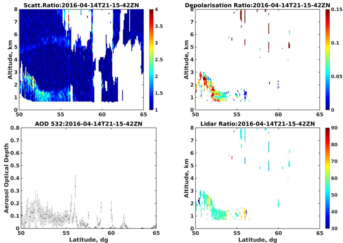
**Figure 14.** Latitudinal cross-section of CALIOP 532 nm scattering ratio  $R_{532}$  (top left), aerosol depolarization ratio  $\delta_{532}$  (top right), aerosol optical depth  $AOD_{532}$  (bottom left) and lidar ratio  $S_{532}$  (bottom right) for 14/4/2016.
