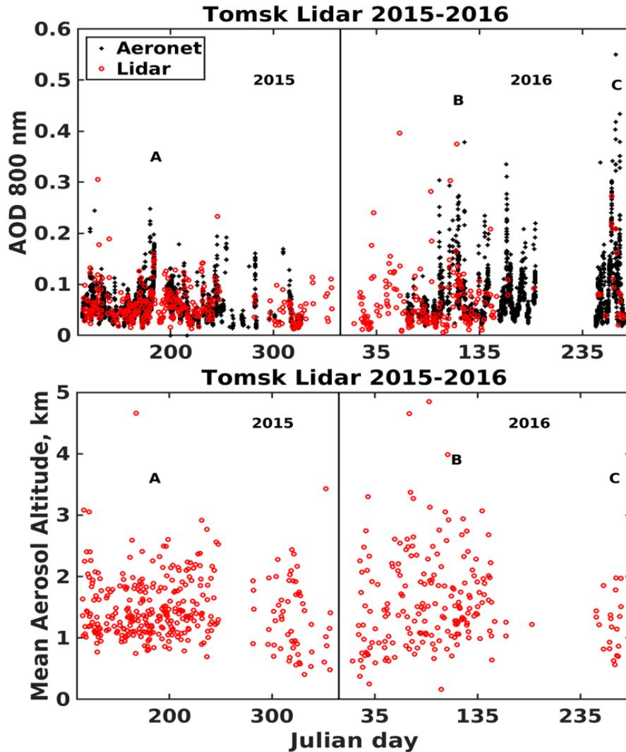
**Figure 8.** Time evolution from April 2015 to September 2016 of the 808 nm AOD for lidar (red) and sun-photometer (black) observations (upper panel) and corresponding aerosol altitudes  $z_{aer}$  given by Eq. 2 (bottom panel). A, B, and C are the cases analyzed in section 5
