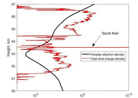
Figure 7. Electron density measured with the Faraday instrument, and the total dust charge density as observed by DUSTY, on MXD-1.
