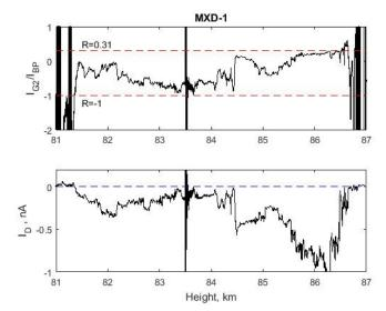
Figure 2. The ratio of the currents to G2 and BP in the upper panel, compared to the current  $I_D$  in the lower panel. The large disturbance at ~ 83.5 km altitude is caused by a squib being fired to open for another experiment on the payload. The values of R, at and outside the borders of the cloud are to be neglected since the dust density there is low or zero and R is therefore dominated by noise and uncertainties in their background level.
