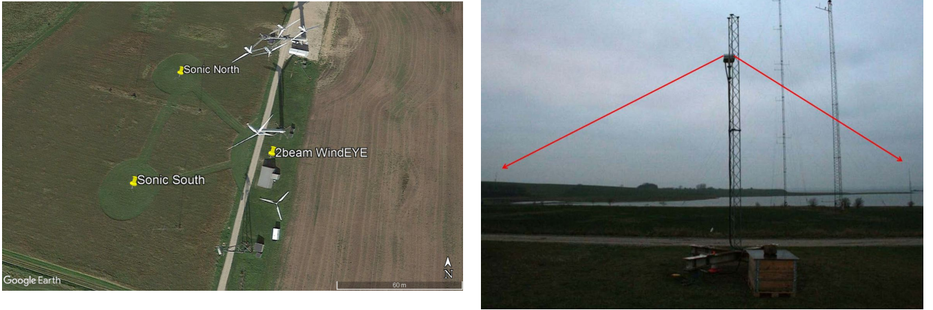
Figure 2. Left: Google Earth screen shot of the site setup. Right: Photo depicting the lidar mounted on the mast looking at the two sonic anemometers, Dellwik et al. (2015)
