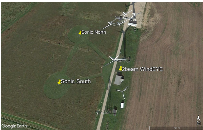
Figure 2. Left: Google Earth screen shot of the site setup. Right: Photo depicting the lidar mounted on the mast looking at the two sonic anemometers, Dellwik et al. (2015)
