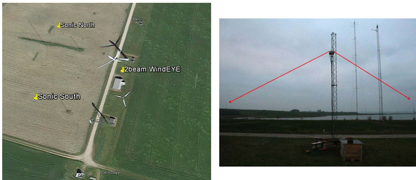
Figure 2. Left: Photo depicting the lidar mounted on the mast looking at the two sonic anemometers, Dellwik et al. (2015). Right: Google Earth screen shot of the site setup
