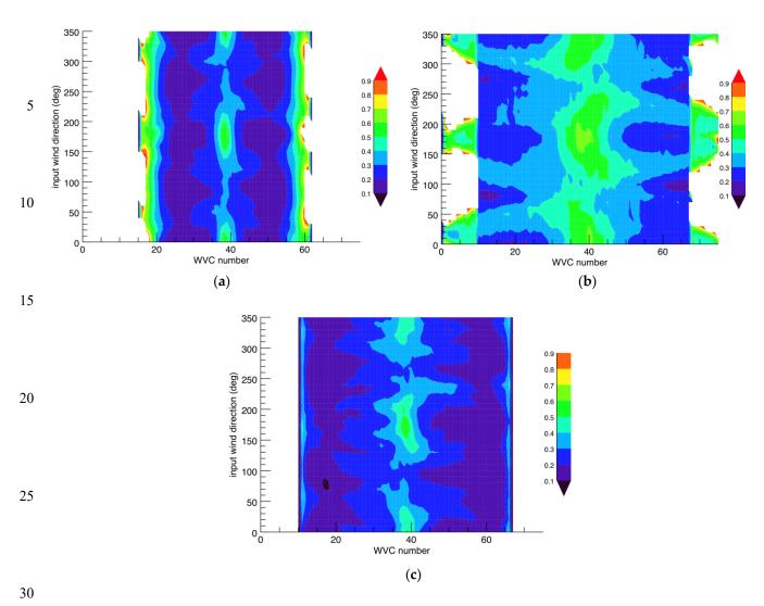
Figure 17: FoM VRMS map as a function of across-track location and wind direction (wind speed is 9 m/s). (a) SCAT; (b) SeaWinds; (c) WindRad.
