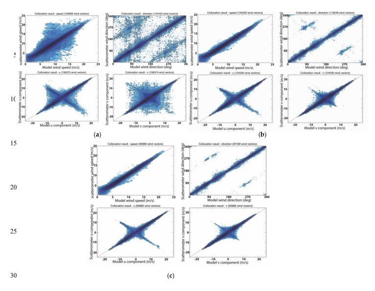
Figure 13: Contoured histograms of SCAT retrieved 1st rank wind solution versus input wind field for 4 orbits. (a) all WVCs within the swath; (b) excluding the WVCs in the outer swath, WVC number from 8 to 42 are included; (c) excluding the WVCs in the outer swath and nadir swath, WVC number from 8 to 17 and 26 to 42 are included. From (a) to (c), upper left: wind speed; upper right: wind direction; lower left: u component; lower right: v component. The contour lines are logarithmic.
