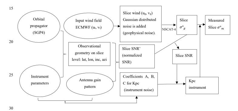
Figure 3: The workflow for generating L1B simulation data.
