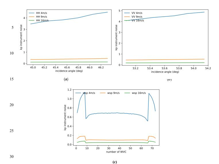
Figure 9: SeaWinds instrument noise in ratio (1 is 100%) at 4m/s, 9m/s, and 16 m/s on (a) slice level of Ku-band HH pol; (b) slice level of Ku-band VV pol (slices with SNR < 0.05 are excluded); (c) WVC mean Kp.
