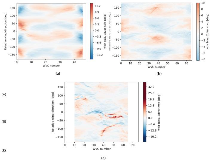
Figure 18: Wind direction bias between wind retrieval result and true wind as a function of WVC number and the relative wind direction (y-axis, the retrieved wind direction relative to the satellite motion direction; color scale is consistent for easy comparison, all the values outside [-20, 20] are marked as dark blue and dark red). (a) SCAT; (b) SeaWinds; (c) WindRad.
