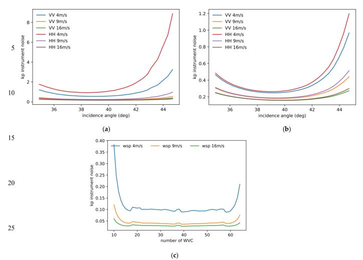
Figure 8: WindRad instrument noise in ratio (1 is 100%) at 4m/s, 9m/s, and 16 m/s on (a) slice level of Ku-band; (b) slice level of C-band (slices with SNR < 0.05 are excluded); (c) WVC mean Kp.
