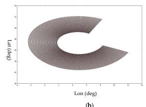
(a) (b) Figure 5: (a) One simulated satellite orbit for CFOSAT starting from 11-12-2011 with the circular motion of the slice located at the end of each pulse; (b) the zoomed in location of all slices on the earth.
