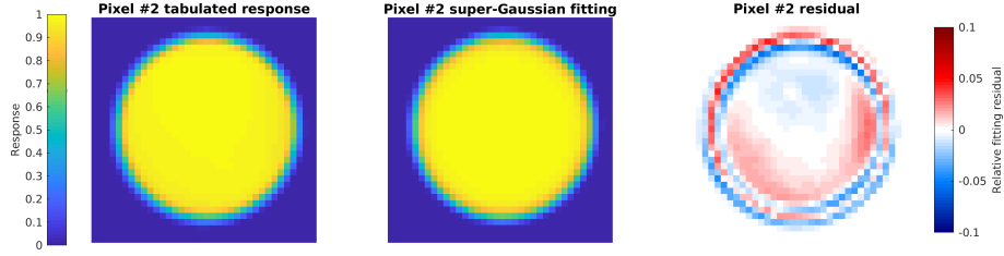
Figure A2. Fitting a tabulated IASI spatial response function for pixel #2 using rotating super Gaussian. The fitted exponent is 18.5.
